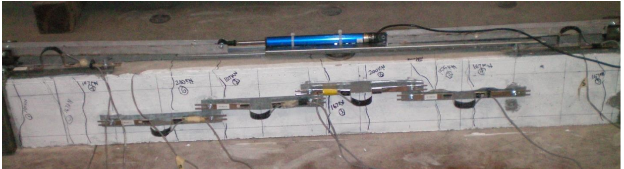
Figure 4.58 Crack Pattern of Strap 45% I-B
