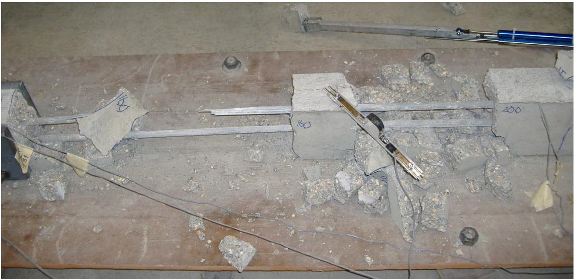
Figure 3.16 Failure of GFRP Prestressed Concrete Strap
