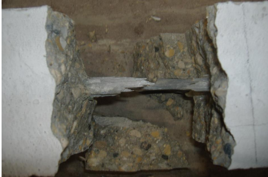
Figure 4.43 Failure Mode of Strap 55% I-A
