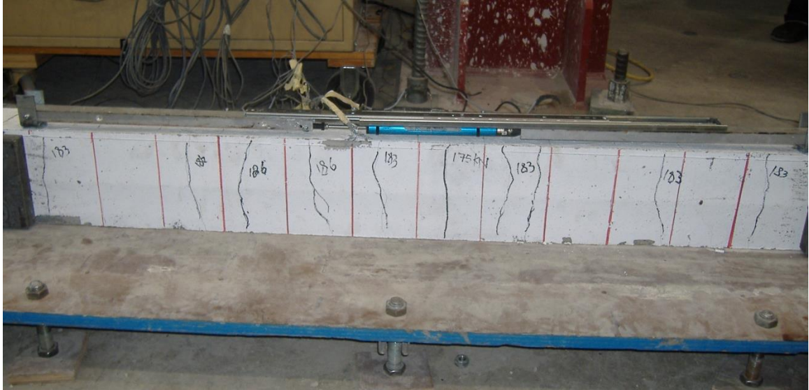
Figure 4.32 Crack Propagation of Strap 35% I-A
