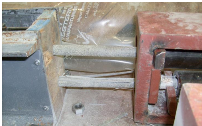
Figure 4.4 Rupture of GFRP After Prestressing
