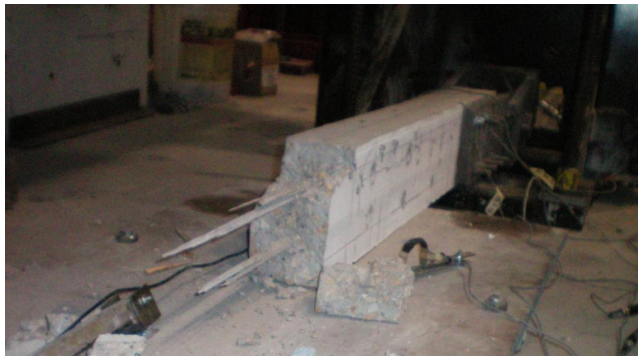
Figure 4.53 Failure Mode of Strap 35% I-B
