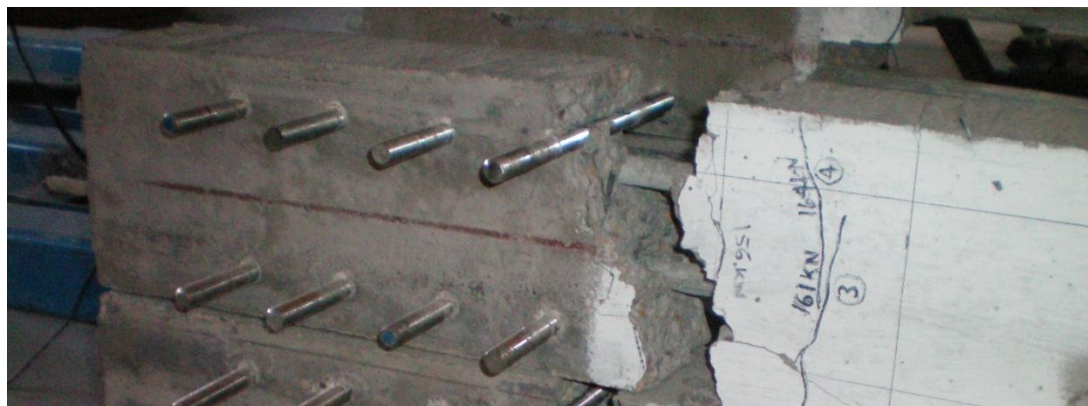
Figure 4.61 Failure Mode of Strap 45% II-B
