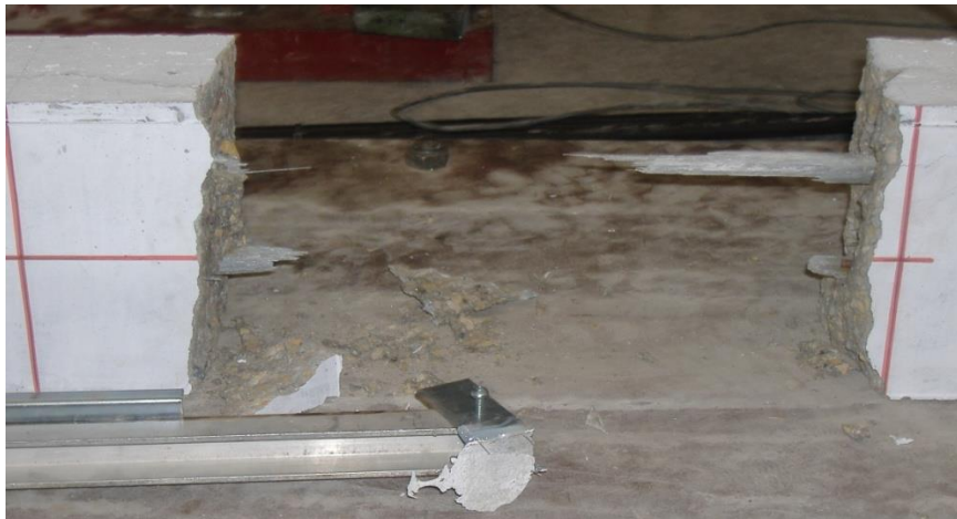
Figure 4.43 Failure Mode of Strap 55% I-A
