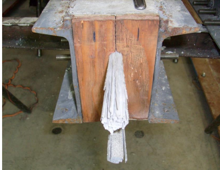
Figure 4.5 Rupture of GFRP After Casting
