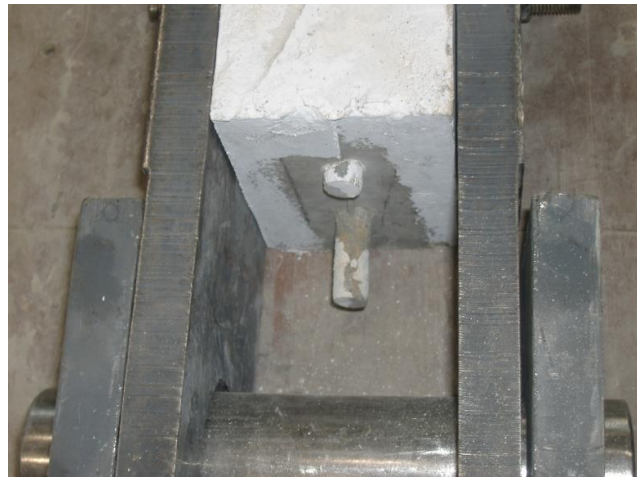
Figure 4.41 Failure Mode of Strap 45% III-A
