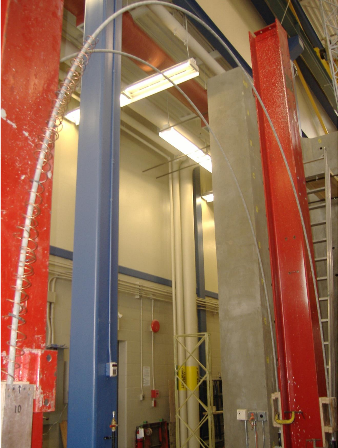
Figure 4.2 GFRP Bars Bent for Casting of Anchorage.
