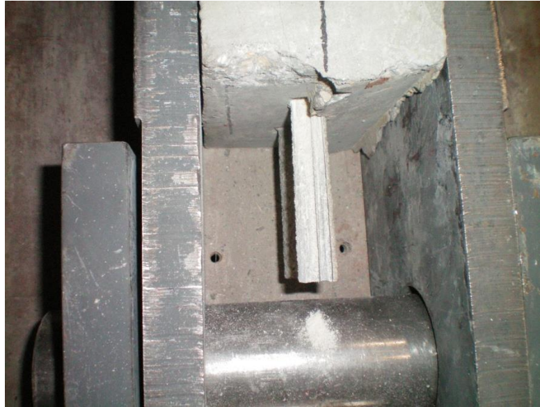
Figure 5.60 Failure Mode of Strap 45% I-B
