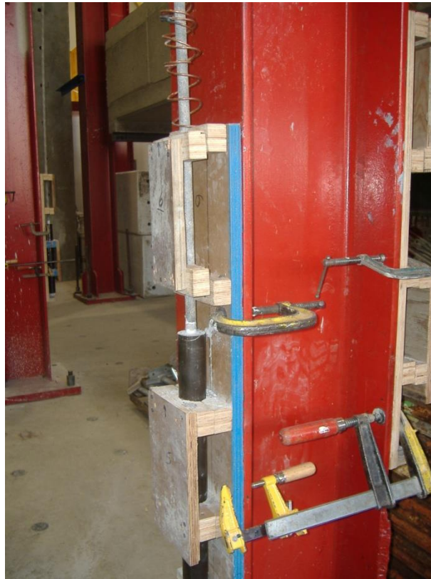
Figure 4.1 Wooden Jig Alligning the GFRP Bar in Steel Anchor Sleeves.
