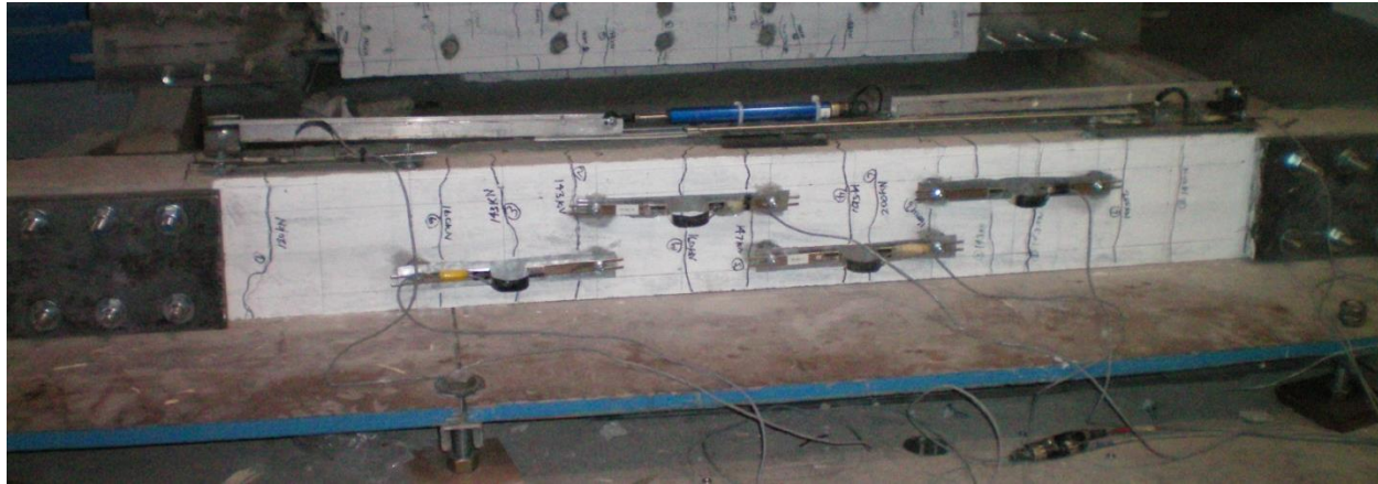
Figure 4.54 Crack propagation of Strap 35% II-B
