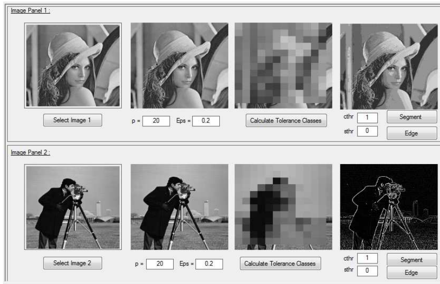
Figure 18: Examples of segmentation and edge detection in the GUI
