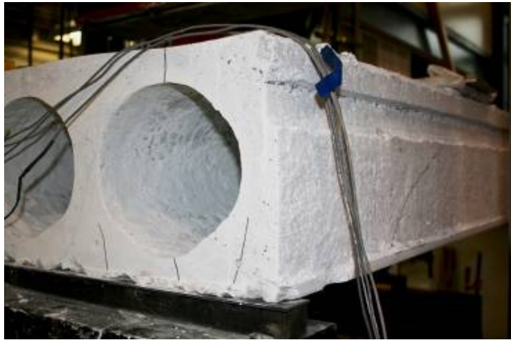
Figure G61: Initial Cracking at Web #5
