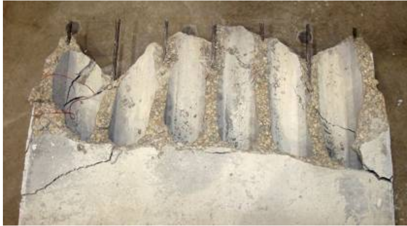
Figure G48: Failure Surface – Plan View (Web #1 on Far Right)
