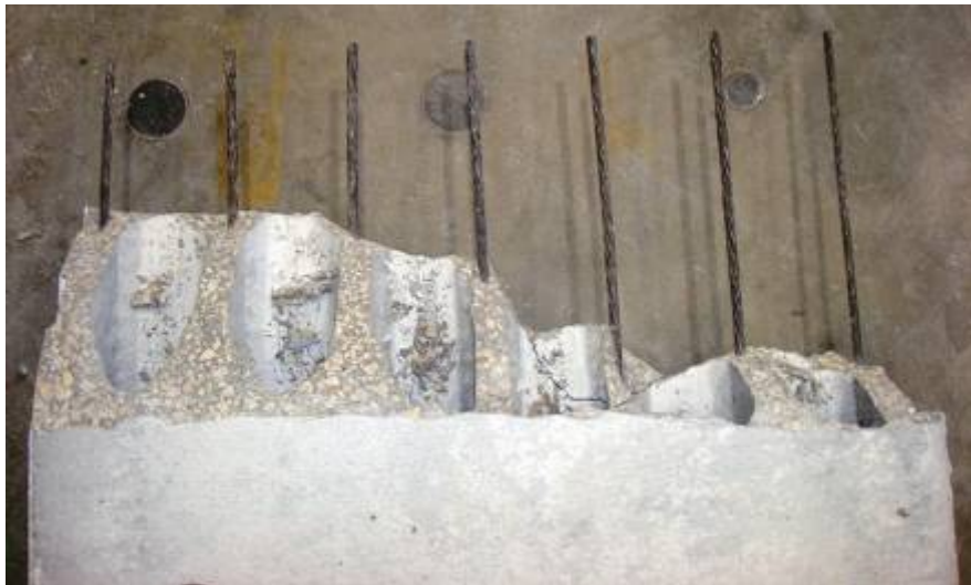
Figure G39: Failure Surface – Plan View (Web #1 on Far Right)
