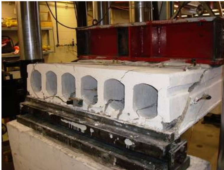
Figure G47: End View of Slab at Failure
