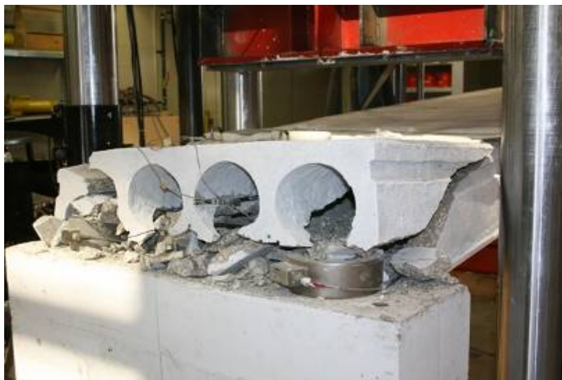
Figure G78: Shear-Tension Failure across Full Slab Width (Web #5 on Far Right)
