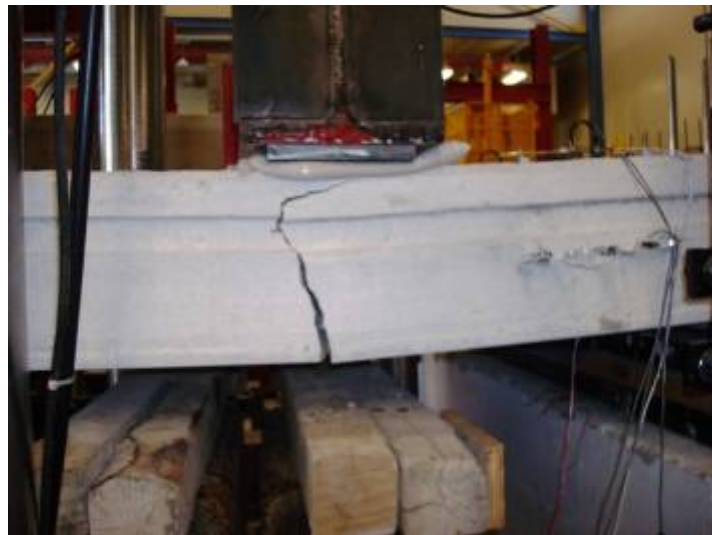
Figure G27: Initial Flexural Crack at Web #1
