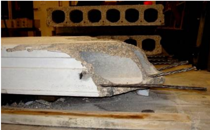
Figure G18: Failure Surface (Web #1 in Foreground)
