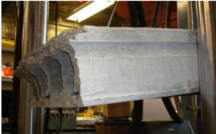
Figure G34: Failure Surface (Web #7 in Foreground)
