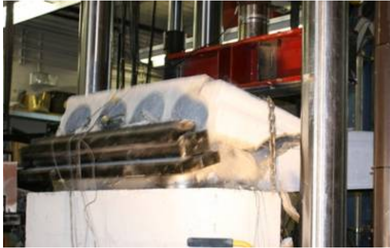
Figure G69: Shear-Tension Failure across Full Slab Width (Web #5 on Far Right)
