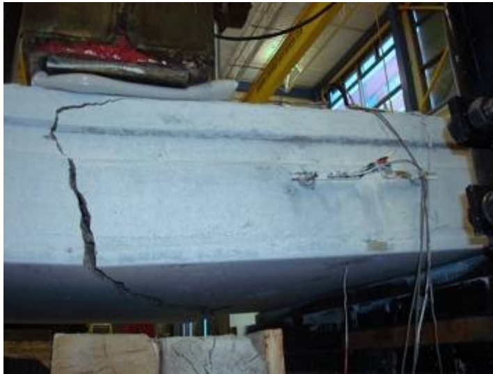
Figure G28: Diagonal Propagation of Crack across Slab Width
