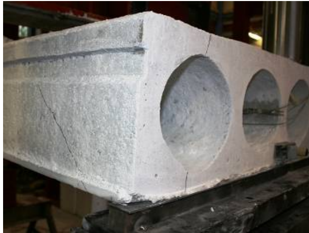
Figure G59: Initial Cracking at Web #1
