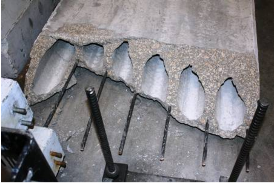
Figure G26: Failure Surface (Web #1 on Far Left)
