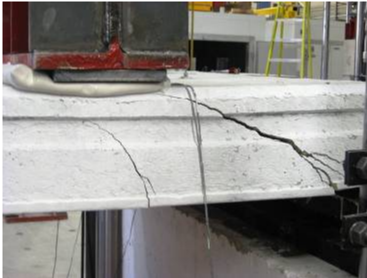
Figure G19: Diagonal Web-Shear Cracks at Web #1 at Failure
