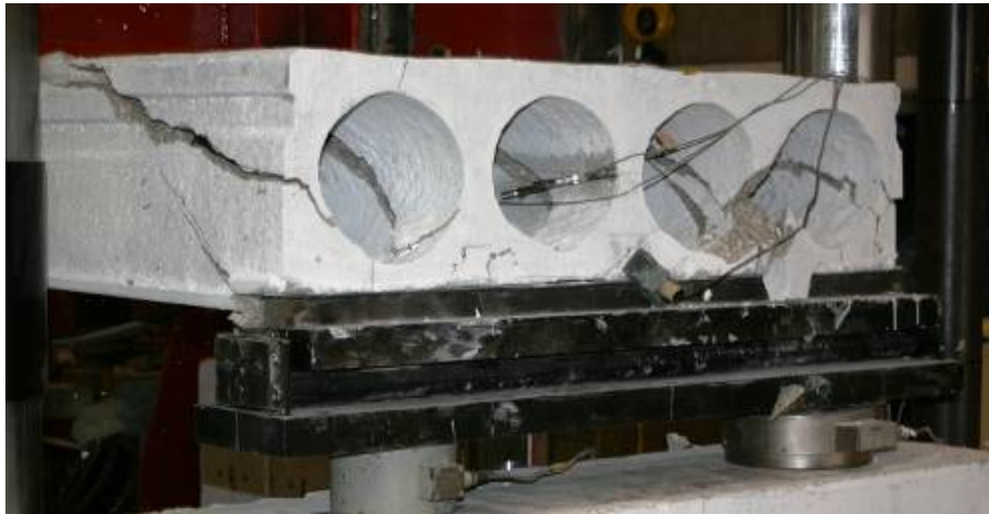
Figure G63: Shear-Tension Failure across Full Slab Width (Web #1 on Far Left)
