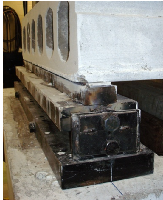
Figure 3.9: Pin Assembly at Loaded End of Test Slab
