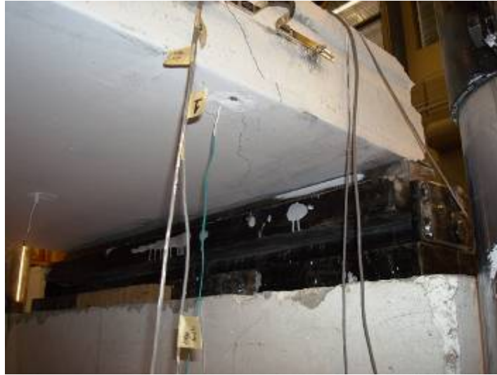
Figure G12: Initial Web-Shear Crack at Web #1 and Diagonal Crack at Slab Underside (92 kN)
