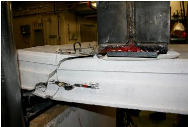
Figure G6: Transition from Flexural to Flexure-Shear Failure at Web #7
