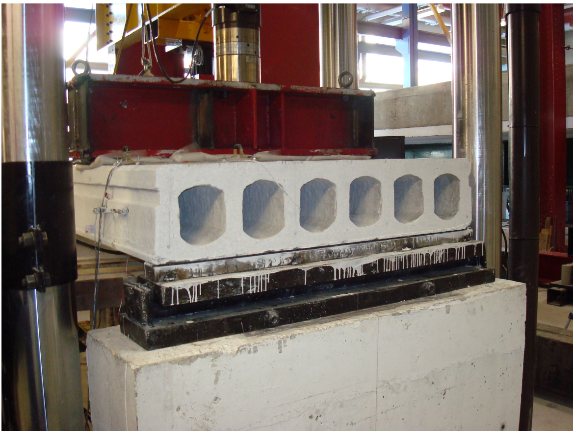
Figure 3.12: Typical Set-up and Instrumentation for Hollow-Core Slab Shear Tests
