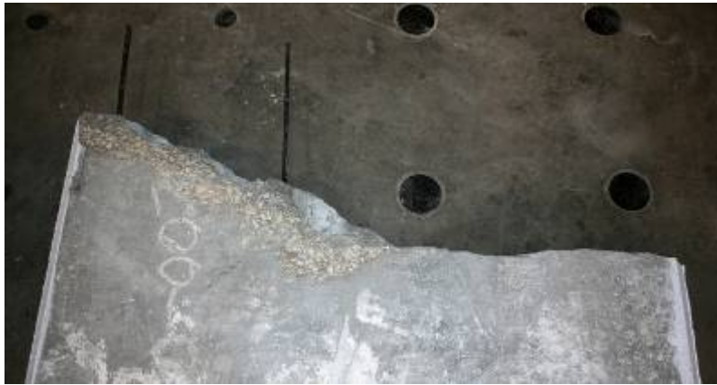
Figure G7: Failure Surface – Plan View (Web #1 on Far Right)
