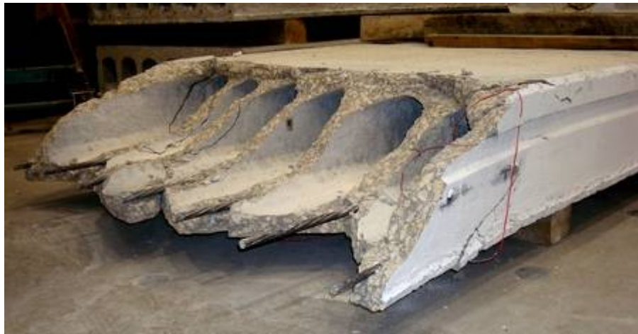
Figure G49: Failure Surface – Elevation View (Web #7 in Foreground)
