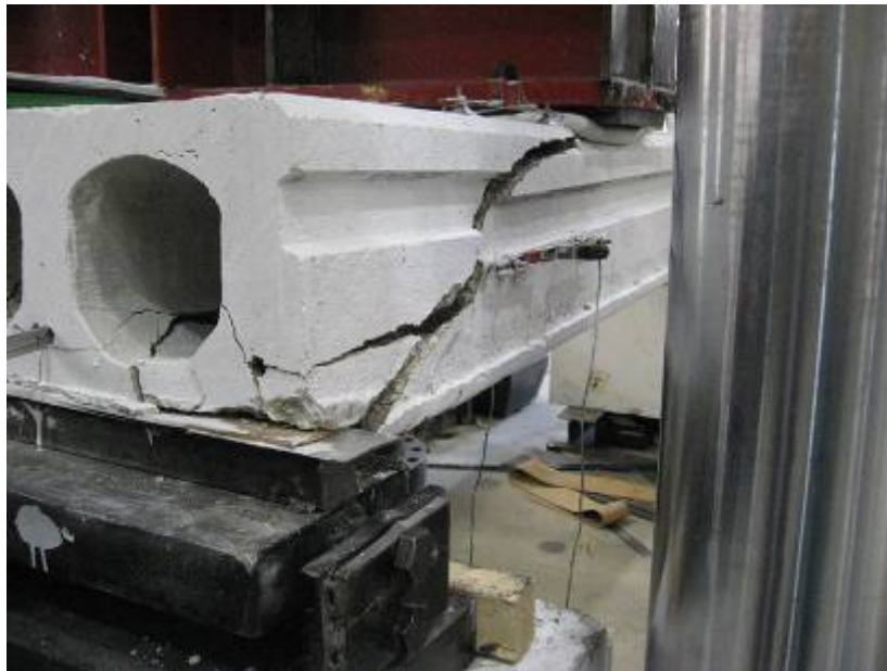
Figure G21: Web-Shear Cracks at Failure (Web #7 in Foreground)
