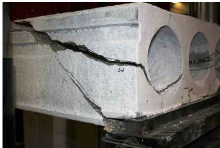
Figure G64: Shear-Tension Failure (Web #1 in Foreground)
