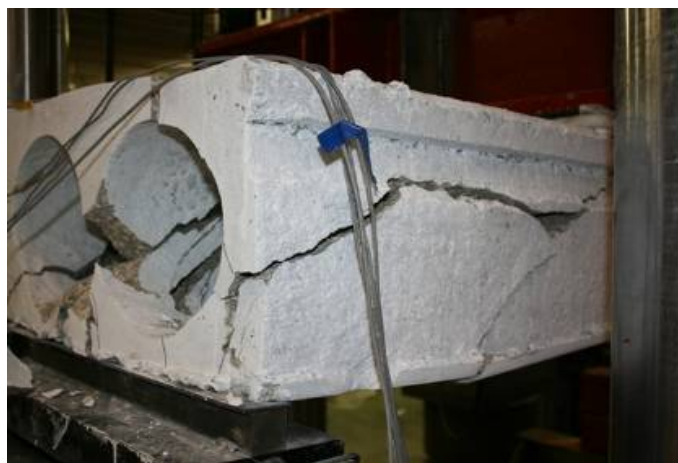
Figure G65: Shear-Tension Failure (Web #5 in Foreground)
