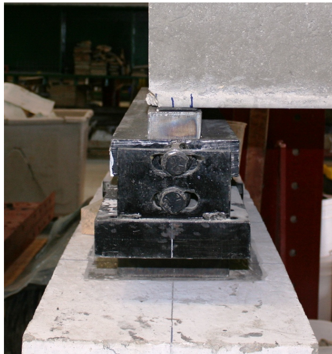
Figure 3.11: Roller Assembly at Opposite End of Test Slab
