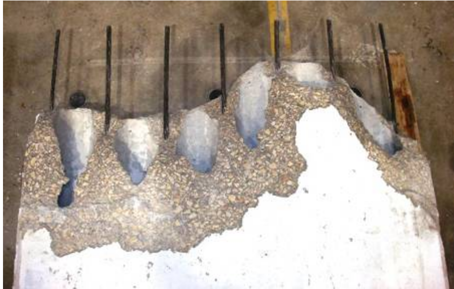
Figure G16: Failure Surface – Plan View (Web #1 on Far Right)
