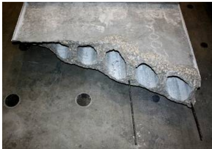
Figure G8: Failure Surface – (Web #7 on Far Right)
