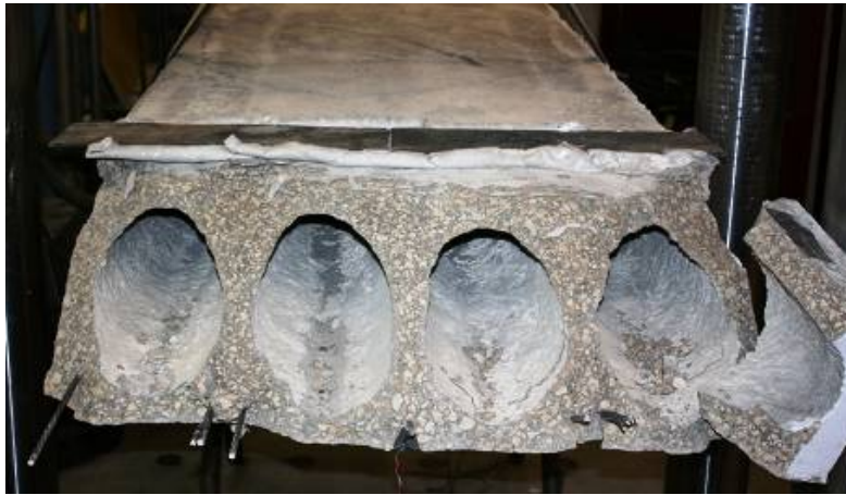
Figure G57: Failure Surface – Elevation View (Web #1 on Far Left)
