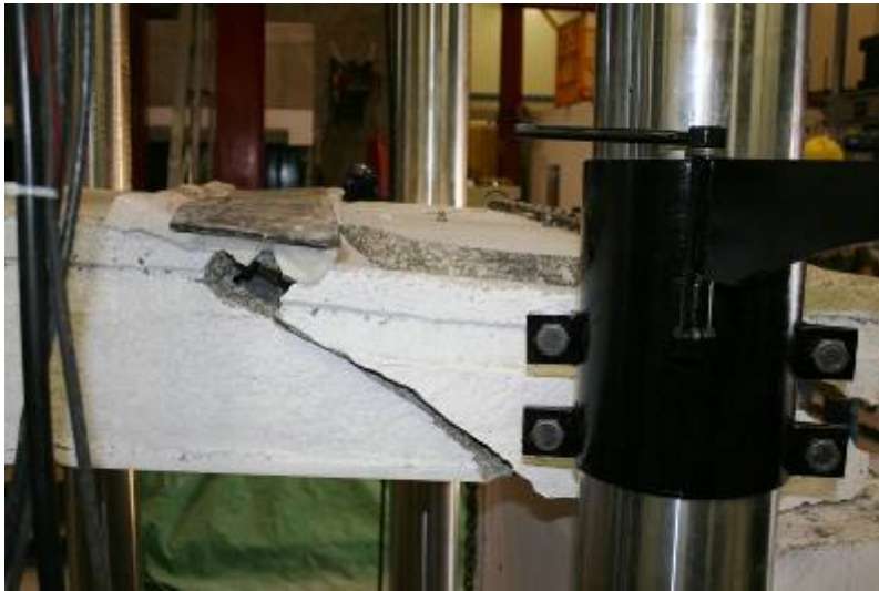
Figure G71: Shear-Tension Failure (Web #1 in Foreground)
