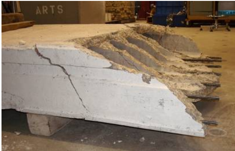
Figure G50: Failure Surface (Web #1 in Foreground)
