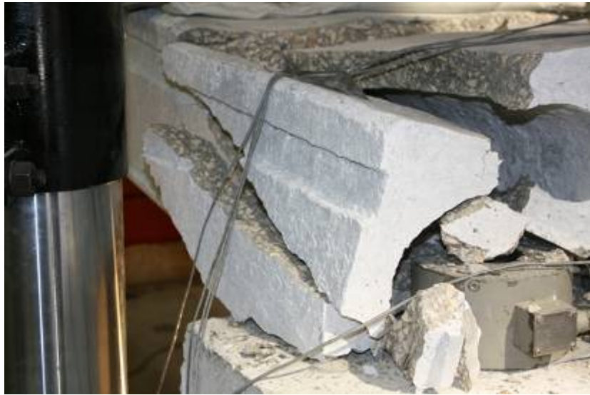
Figure G79: Shear-Tension Failure (Web #1 in Foreground)
