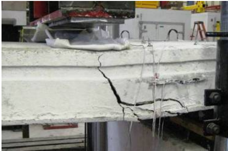
Figure G36: Initial Crack and Shear Tension Failure at Web #1
