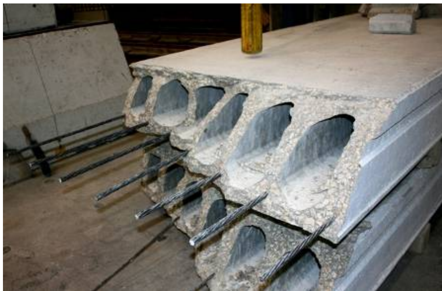
Figure G41: Failure Surface – Elevation View (Web #7 in Foreground)
