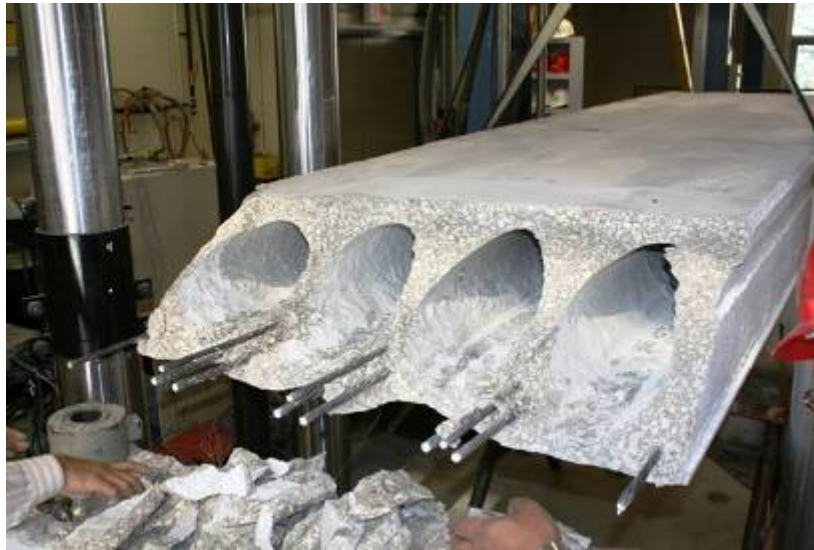
Figure G81: Failure Surface – Elevation View (Web #5 on Far Right)
