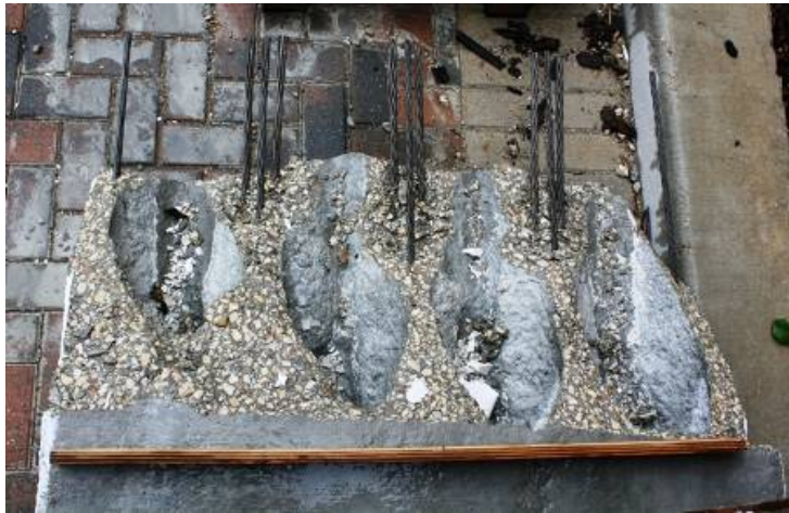
Figure G73: Failure Surface – Plan View (Web #1 on Far Right)
