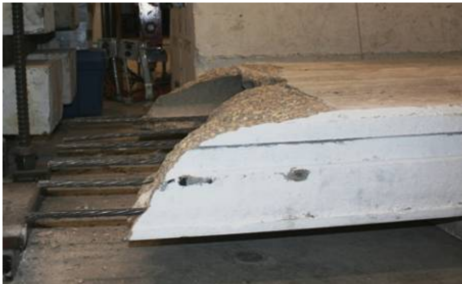
Figure G25: Failure Surface – Elevation View (Web #7 in Foreground)
