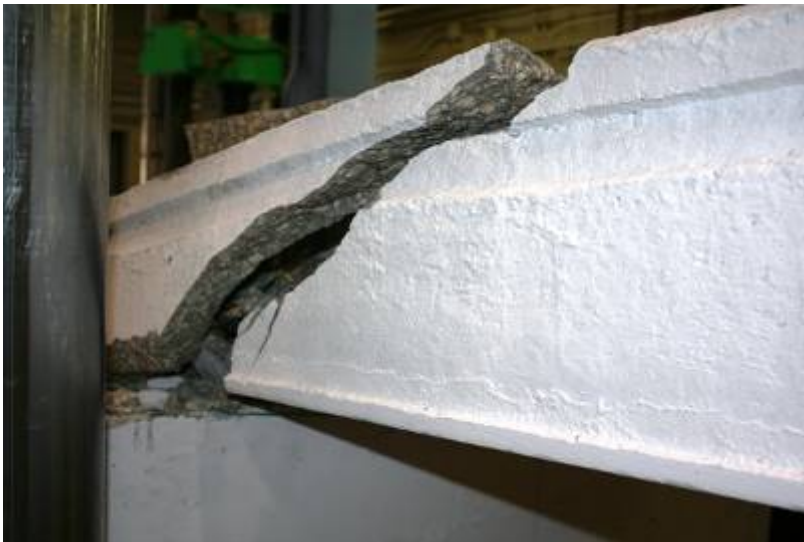
Figure G72: Shear-Tension Failure (Web #5 in Foreground)
