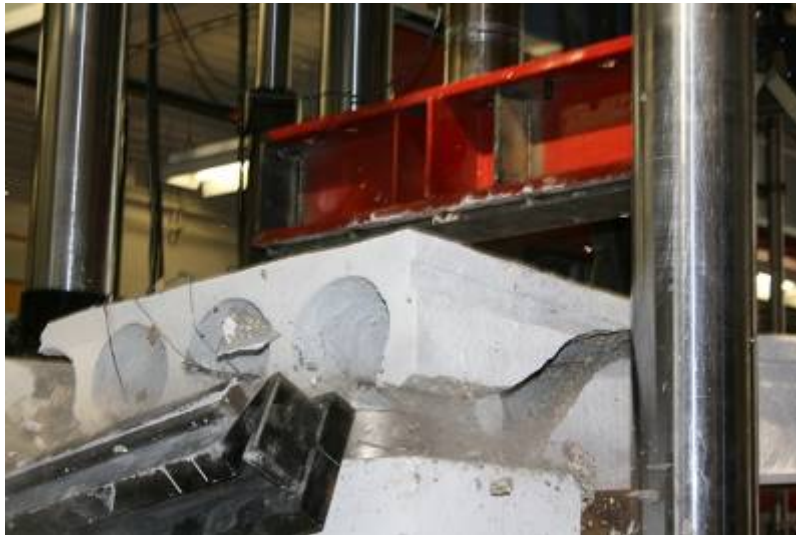
Figure G77: Shear-Tension Failure across Full Slab Width (Web #5 on Far Right)
