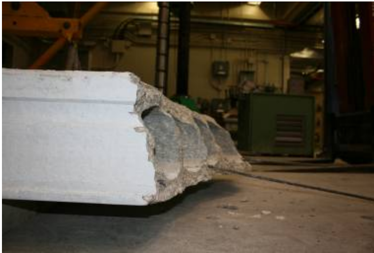
Figure G32: Failure Surface (Web #1 & Ruptured Strand in Foreground)
