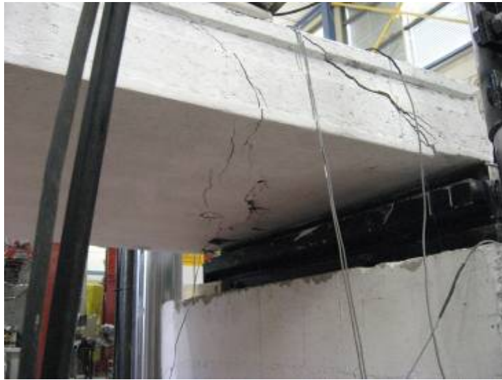
Figure G20: Initial Cracks at Web #1 and Diagonal Crack at Slab Underside
