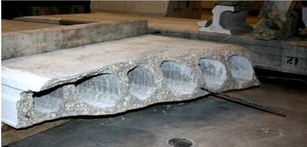
Figure G10: Failure Surface (Web #1 & Ruptured Strands in Web #1 and #3 in Foreground)
