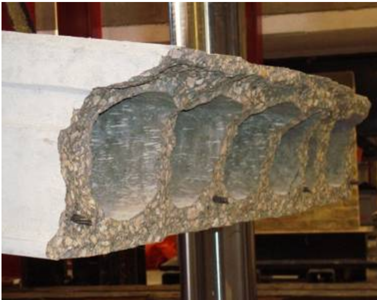
Figure G35: Failure Surface (Web #1 in Foreground)
