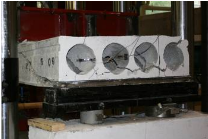
Figure G54: Shear-Tension Failure across Full Slab Width (Web #1 on Far Left)
