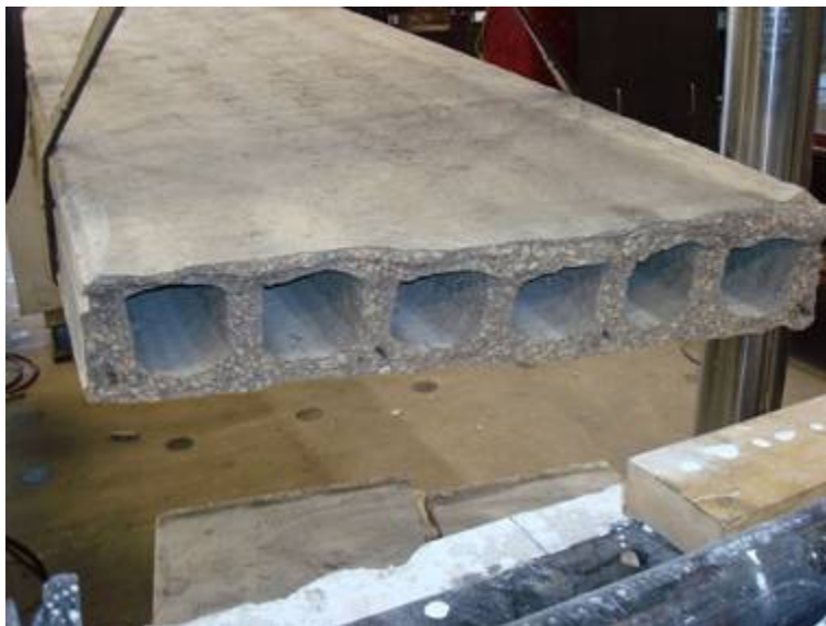
Figure G33: Failure Surface (Web #1 on Far Left)
