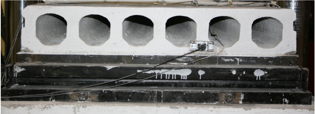
Figure 3.10: Elevation of Pin Assembly at Loaded End of Test Slab
