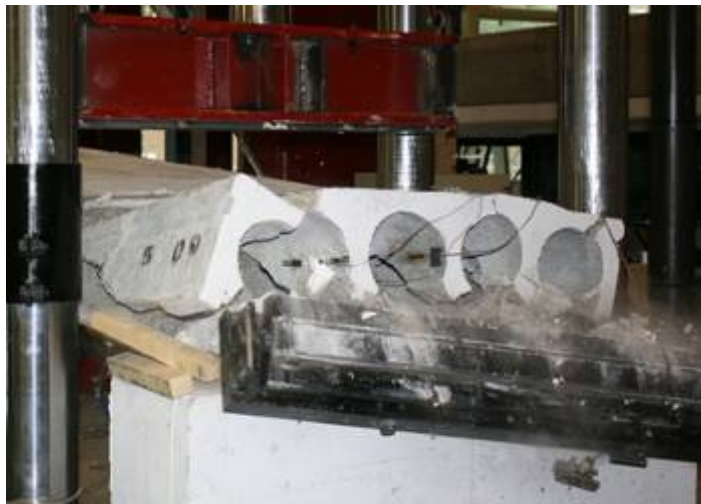
Figure G55: Shear-Tension Failure across Full Slab Width (Web #1 on Far Left)
