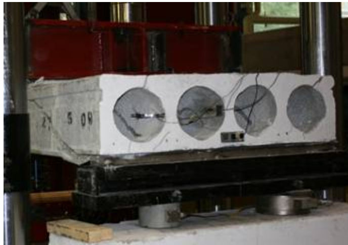
Figure G53: Shear-Tension Failure across Full Slab Width (Web #1 on Far Left)
