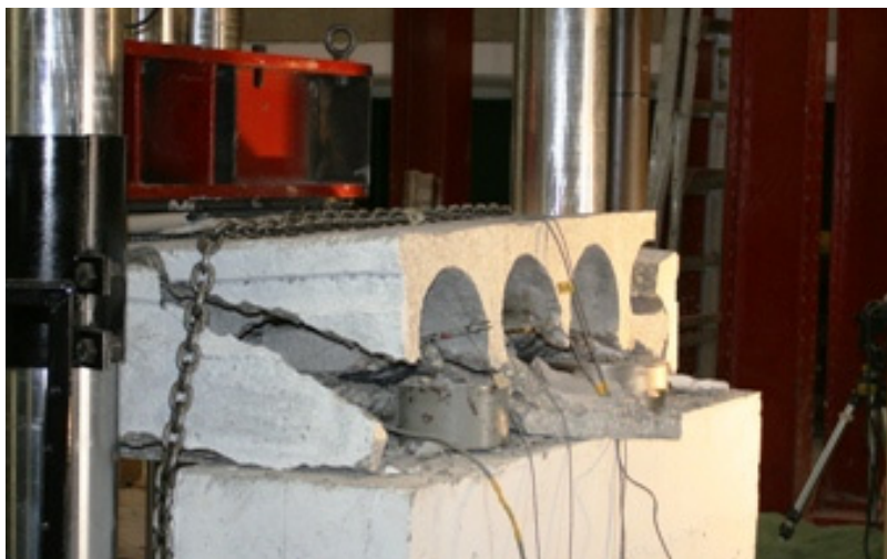
Figure G70: Shear-Tension Failure across Full Slab Width (Web #1 on Far Left)
