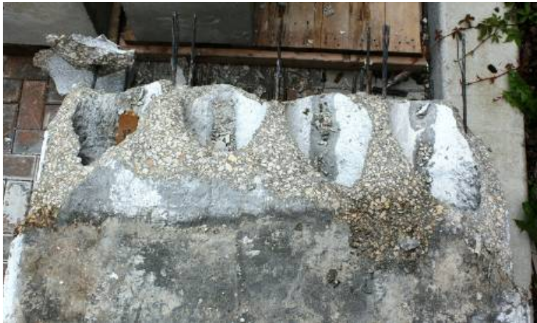
Figure G56: Failure Surface – Plan View (Web #1 on Far Right)
