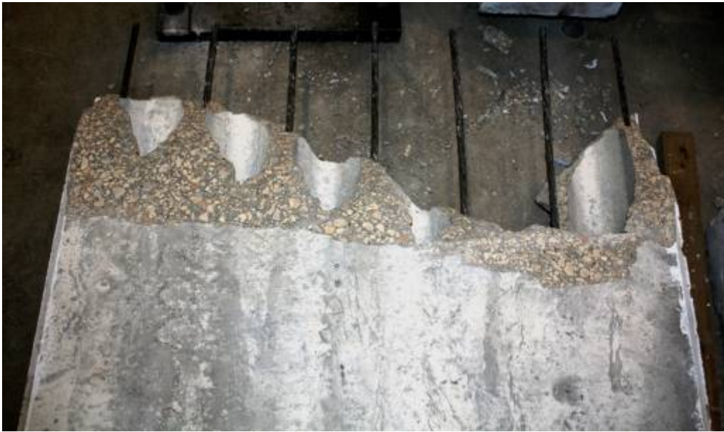
Figure G24: Failure Surface – Plan View (Web #1 on Far Right)
