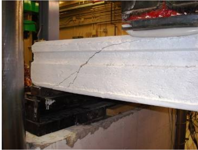
Figure G14: Web-shear Failure across Full Slab Width (Web #7 in Foreground)
