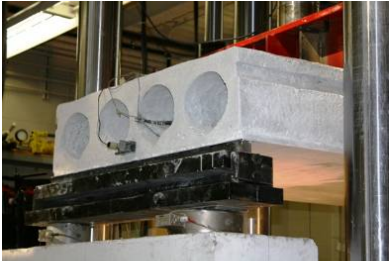
Figure G76: Shear-Tension Failure across Full Slab Width (Web #5 on Far Right)
