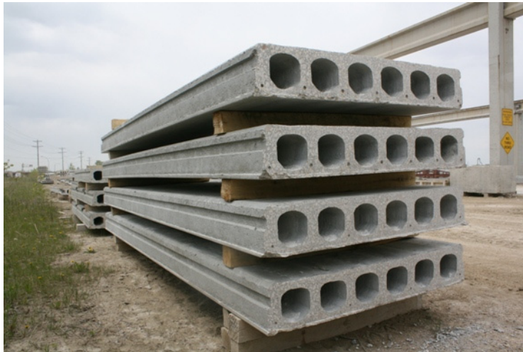
Figure 1.1: Precast Hollow-core Slabs (Saw-cut and Ready for Shipment to Project Site)
