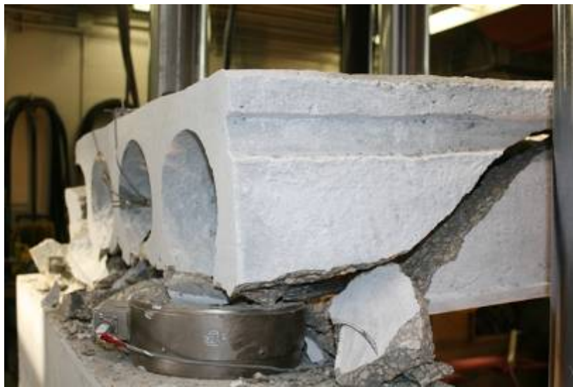
Figure G80: Shear-Tension Failure (Web #5 in Foreground)
