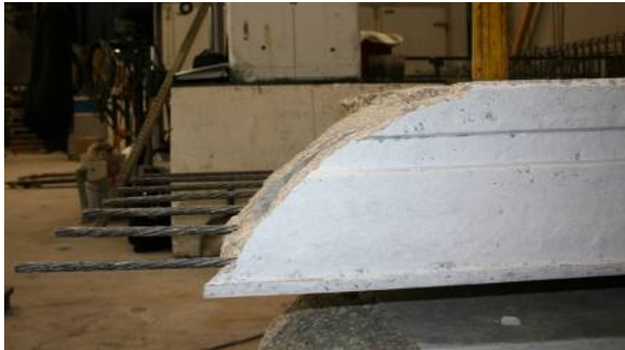
Figure G40: Failure Surface – Elevation View (Web #7 in Foreground)
