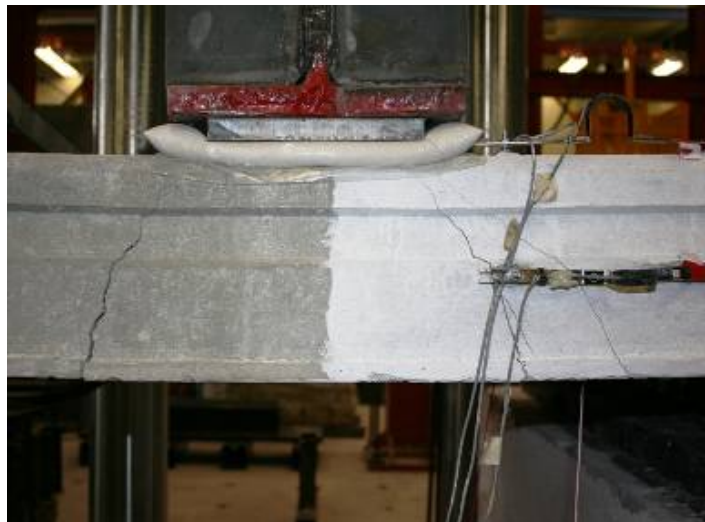
Figure G1: Diagonal Flexure-Shear Cracks at Web #1
