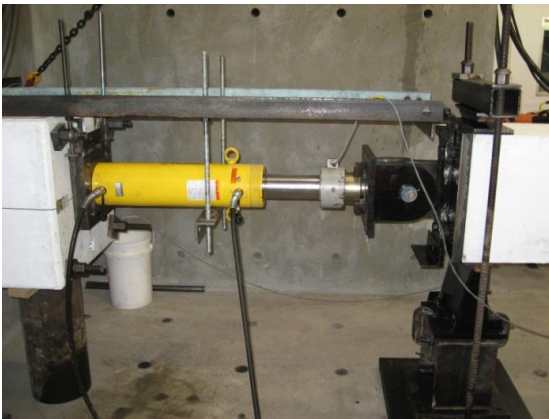
a- Column axial load cell
