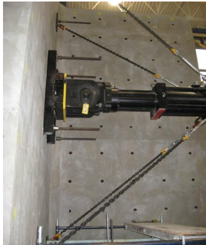
a- Actuator-to-wall connection
