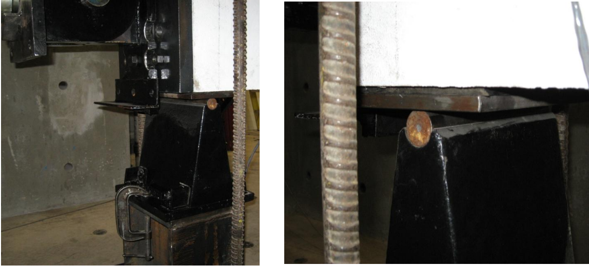
Figure 3.12: Column roller support
