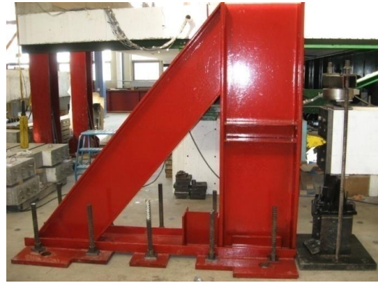
Figure 3.11: Steel reaction frame
