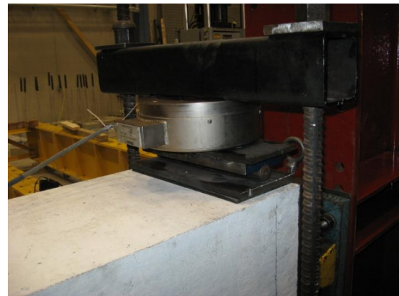
b- Column reaction load cell
