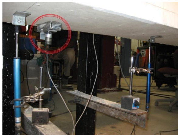
(e) Bar slippage
