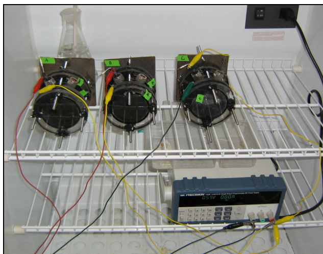
Figure A.1.3 Constructed MECs in operation a) Close-up of reactor without a Ag/AgCl reference probe. b) 3 x MEC experimental set-up with rectifier inside the incubator, next to the c) LabJack data acquisition system.
