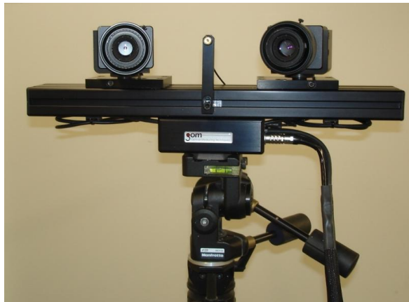
Figure 3.15 – ARAMIS Digital Image Correlation System
