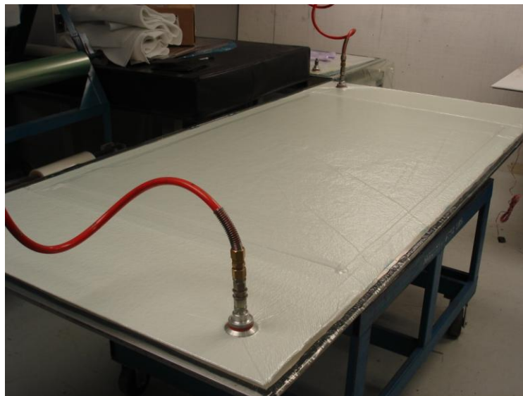
Figure 3.2 – Vacuum Applied During Laminate Manufacture
