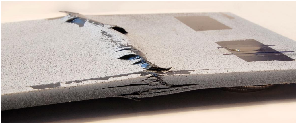
Figure 4.11 – Damaged Specimen After Static Compression Failure
