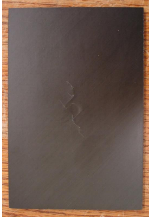
Figure 4.4 – Typical Visible Impact Damage
