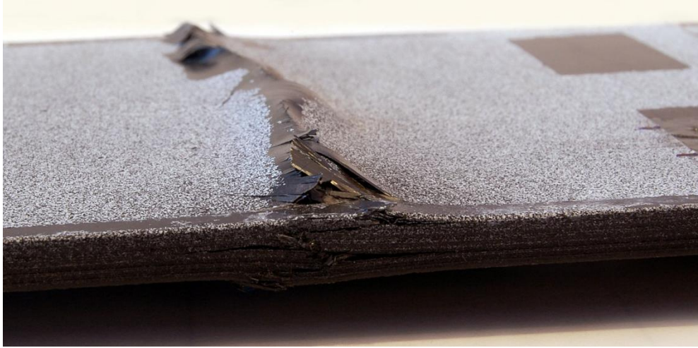
Figure 4.20 – Damaged Specimen After Fatigue Compression Failure
