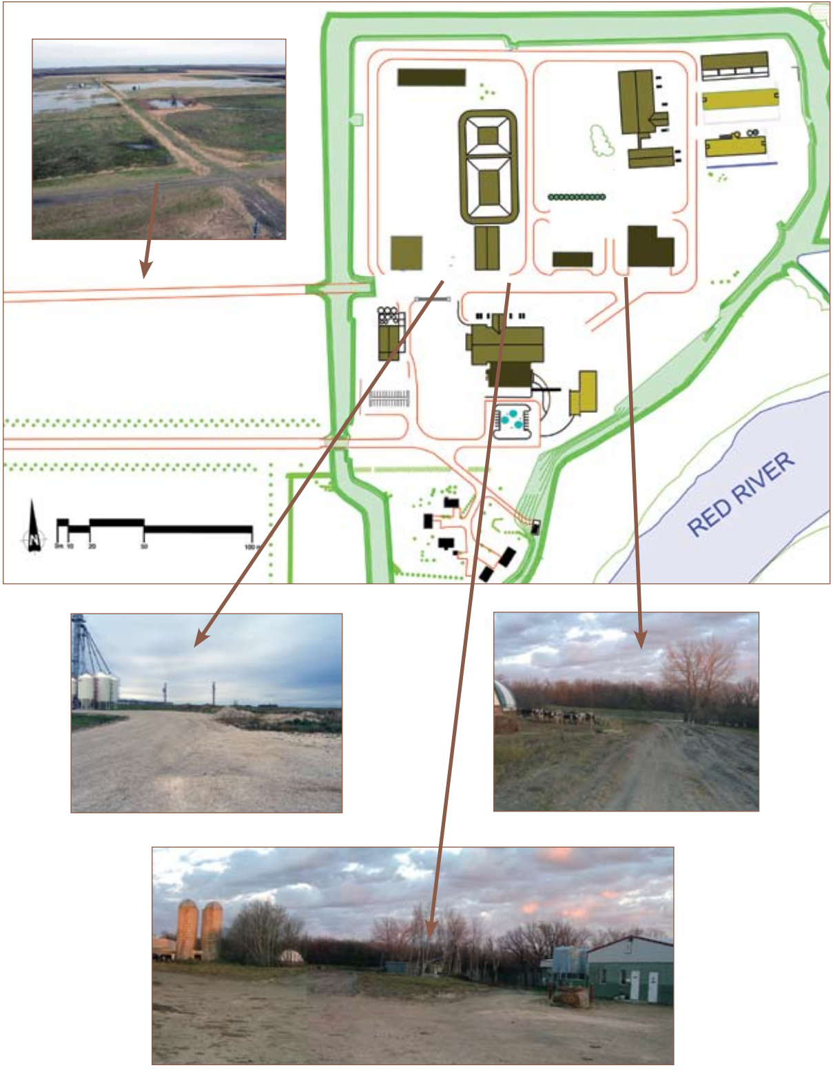
Figure 78: Site circulation. Upper left, the dirt path which provided the foundation for the secondary road in 2010. Lower left, point of entry into the site. Lower right, the new road has not been completed fully to the east. Lower centre, fork for north-south road to lagoon.
