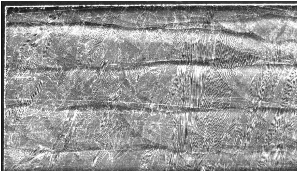
Figure 4.22 – LONGITUDINAL SECTION SHOWING DIFFERENT LAYERS
