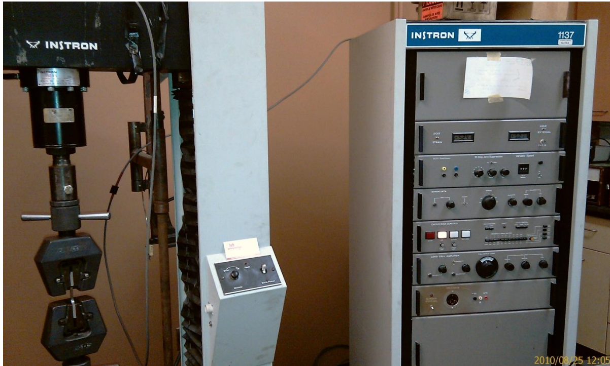
Figure 3.19 – INSTRON TENSILE TESTING EQUIPMENT
