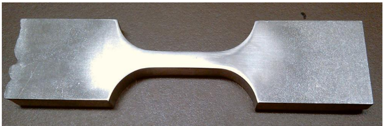
Figure 4.20 – TENSILE TEST SPECIMEN
