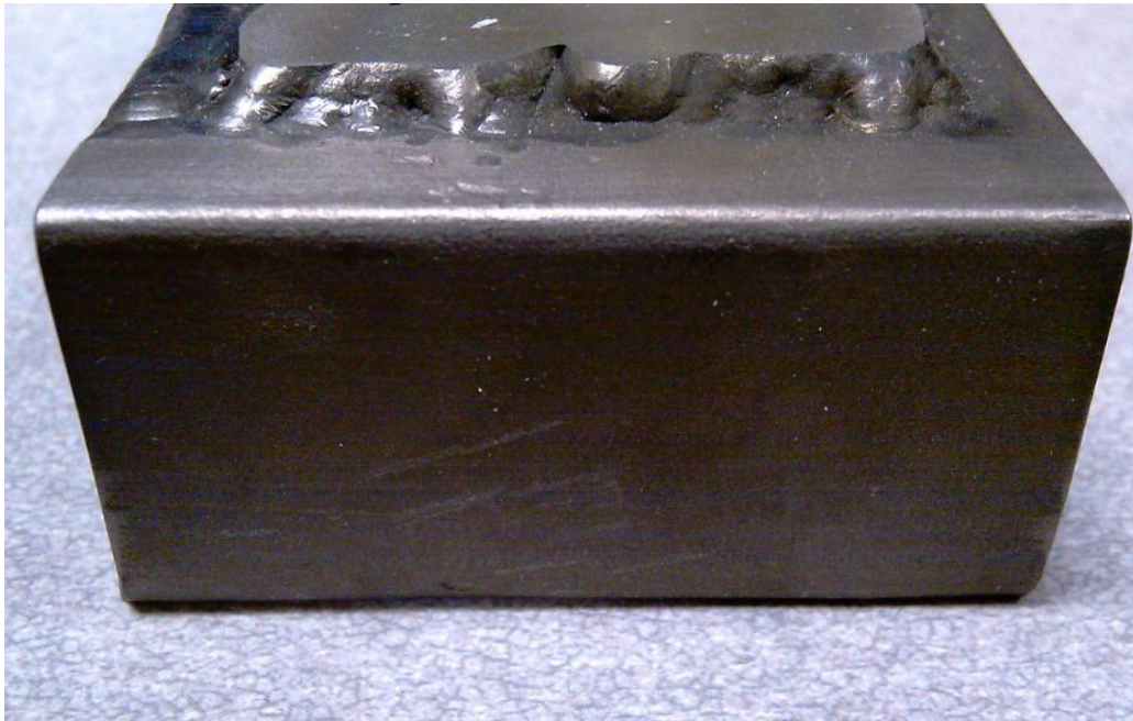
Figure 4.17 – 25 mm THICK BASE AFTER WELDING AND EDM
