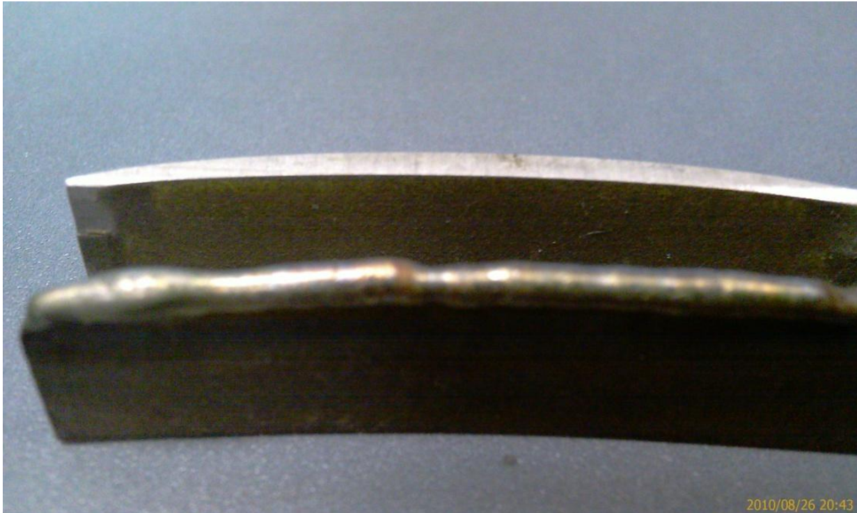
Figure 4.14 – BLADE PROFILE AFTER DEPOSITION OF A LAYER OF METAL
