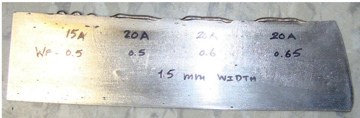
Figure 4.10 – EDGE BUILD-UP 1.5 mm
