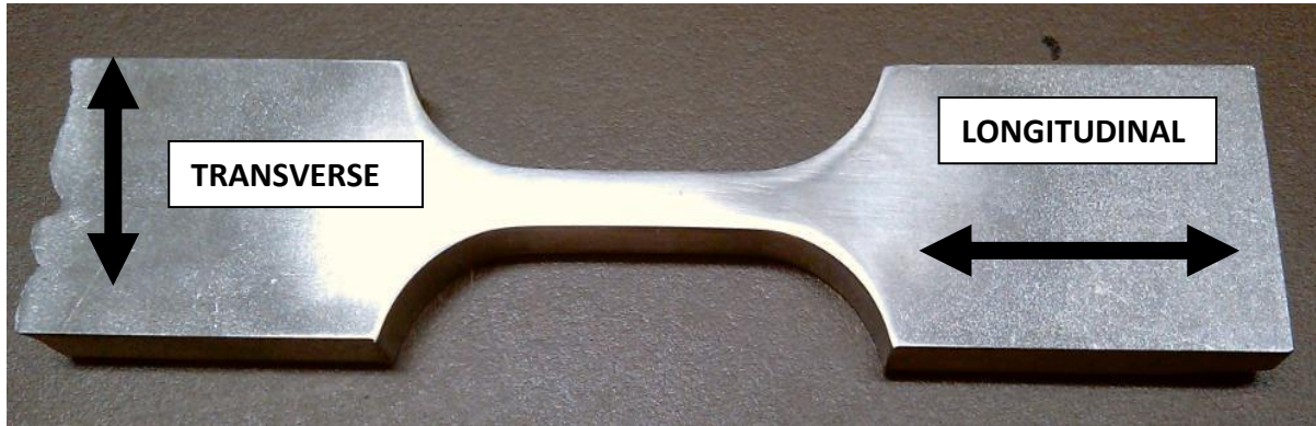
Figure 4.21 – LONGITUDINAL & TRANSVERSE SECTIONS
