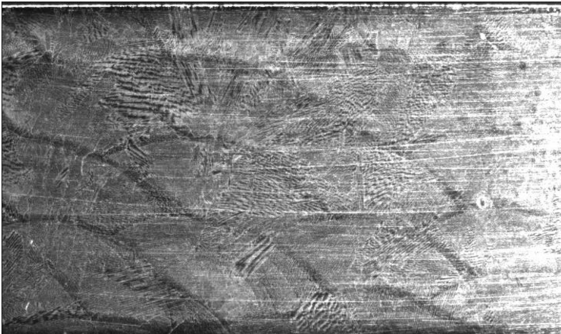
Figure 4.23 – TRANSVERSE SECTION – WELD PASSES & LAYERS
