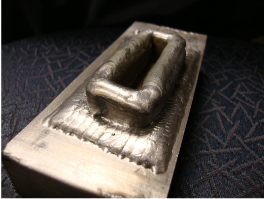
Figure 4.26 – PART – AFTER WELDING
