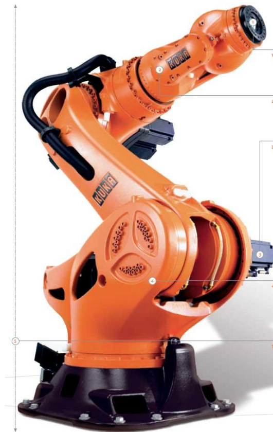
Figure 3.2 – ARTICULATED ROBOT MANUFACTURED BY KUKA [27]
