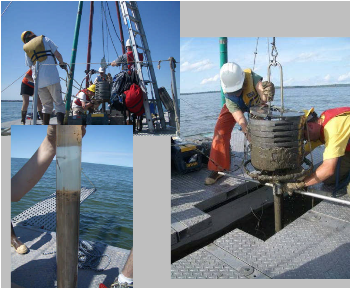
Figure 28. Core recovery operations using the LRC Kullenberg Rig. From top left clockwise: preparing to lower the core barrel and weight assemblies using the hydraulic winch system, recovering the core barrel and weight assemblies through the moon pool, and view of the sediment water interface through the polycarbonate tube of the muck core (photos by J. Teller).
