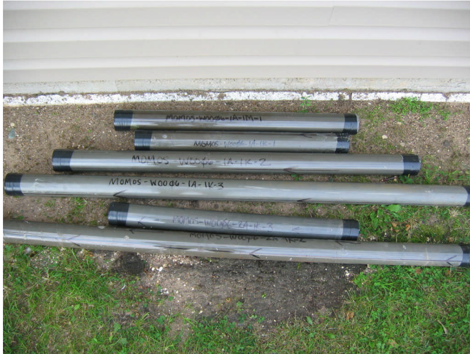
Figure 29. Recovered cores in the polycarbonate liners cut and labeled in preparation for transport.
