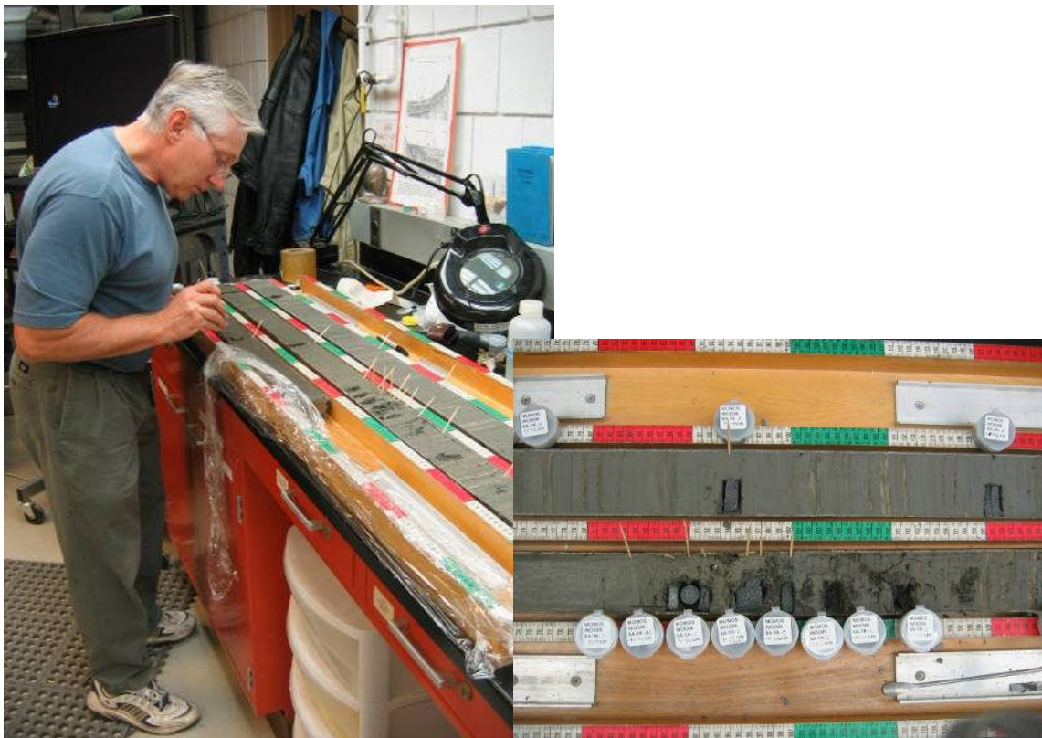
Figure 30. Core subsampling at the LRC of the non-archive half of the split core, using one quarter of the core diameter and the typical subsampling span along the core length of about 2 cm. The subsample plastic sampling containers are shown on the right (photos by J. Teller).
