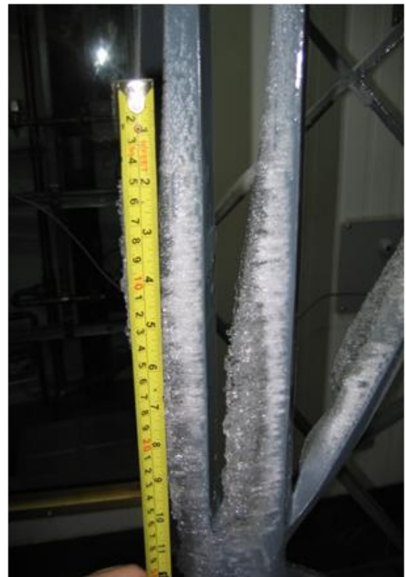
(b) Measured thickness of the glaze ice
