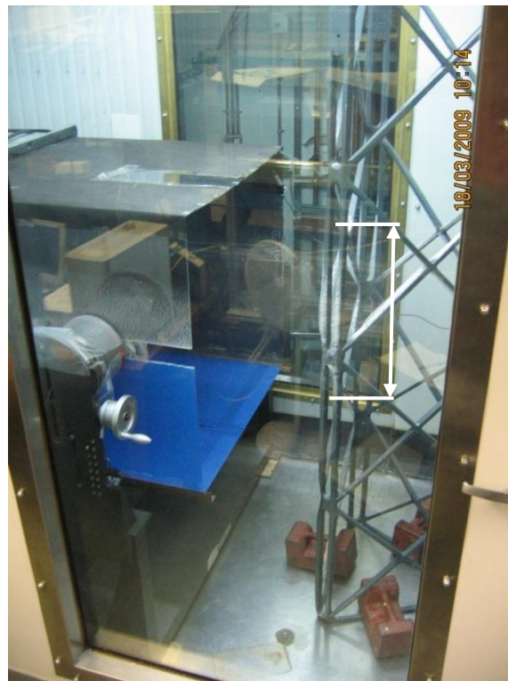
Figure 3.32: Tested segment placed in icing tunnel
