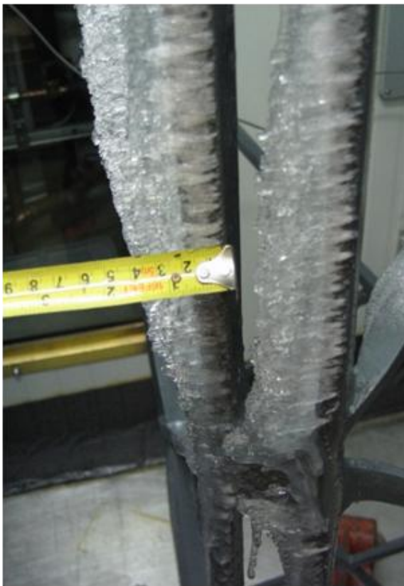
(a) Thickness of the glaze ice
