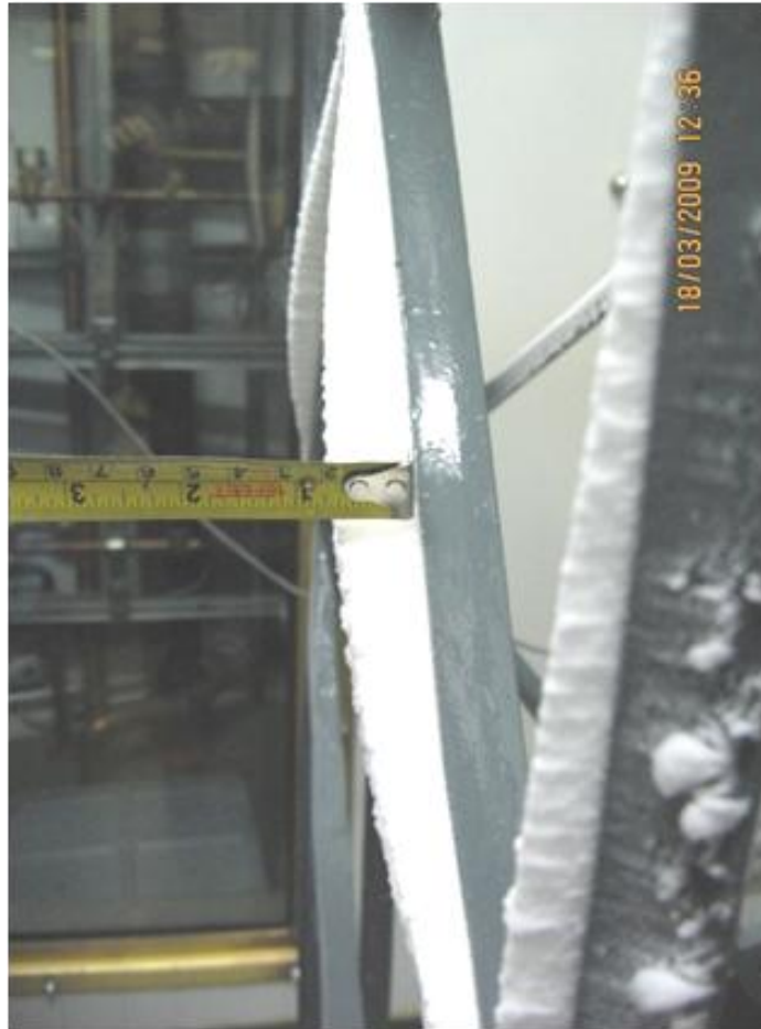
(a) Measured thickness of the soft rime ice
