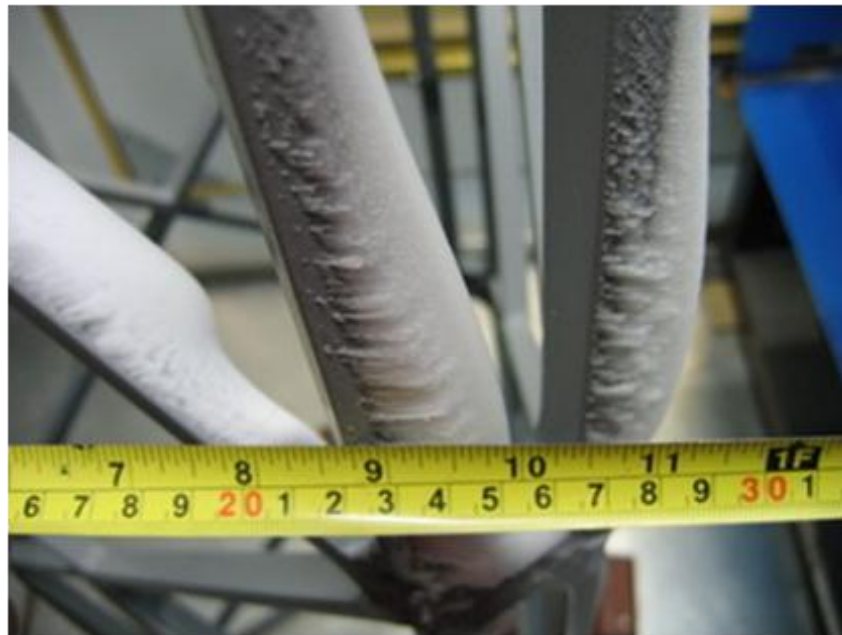
Figure 4.25: Hard rime ice accumulation on the steel tower section coated with Wearlon Super F-1 Ice at 90 degree angle
