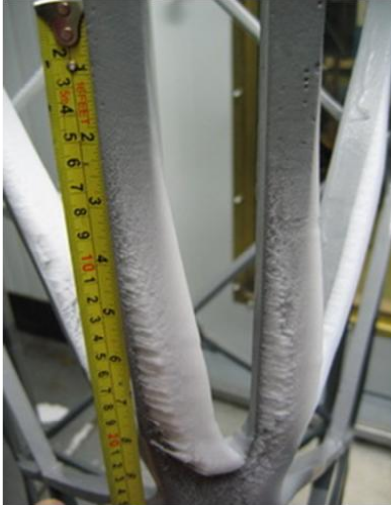
Figure 4.26: Hard rime ice accumulation on the FRP tower section coated with Wearlon Super F-1 Ice at 90 degree angle
