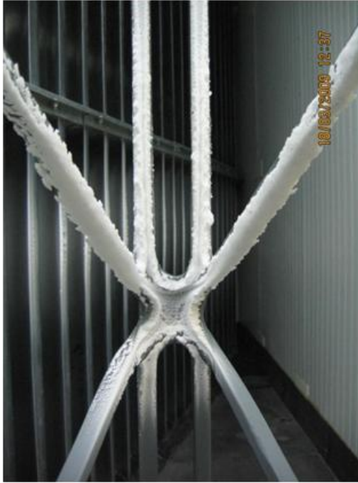
(b) Front view of the iced section
