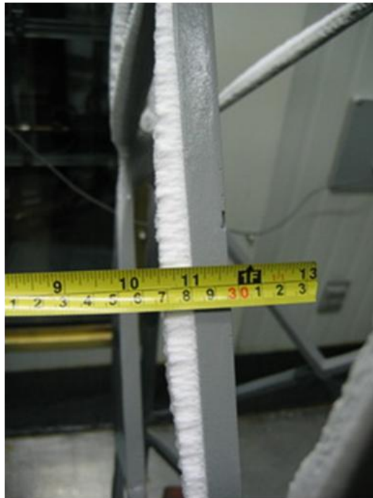
(a) Accretion of the soft rime ice on the diagonal
