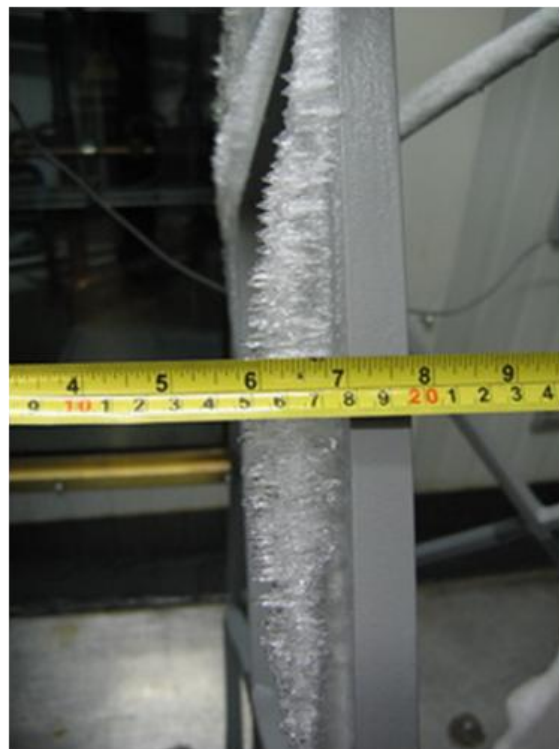
(b) Measured thickness of the glaze ice
