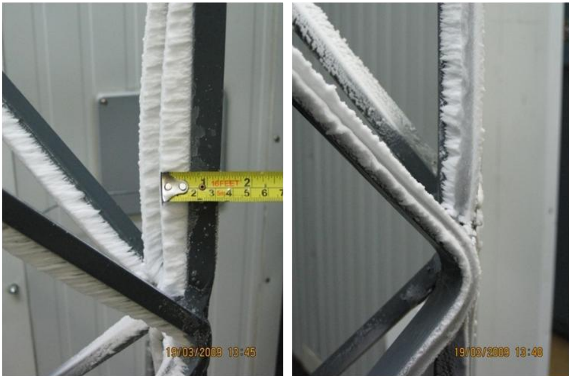
(a) Measured thickness of the soft rime ice
