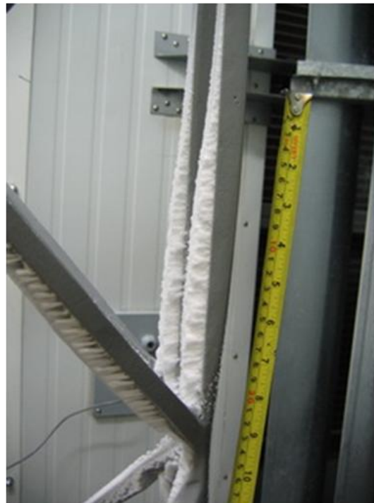
(b) Measured thickness of the soft rime ice on the FRP section
