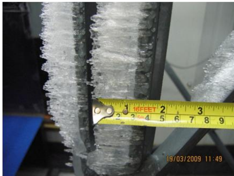
Figure 4.18: Test 4-glaze ice accumulation on the steel tower section at 90 degree angle.
