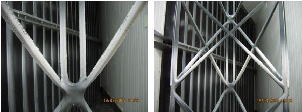
(a) Hard rime ice accretion on chords and diagonals
