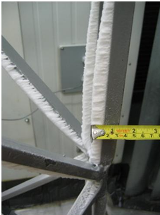
(b) Measured thickness of the soft rime ice on the steel section
