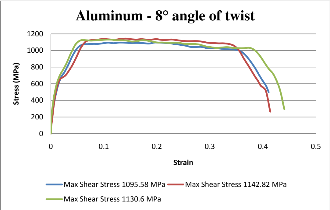
Figure 4.11: Stress-strain curves for Aluminum 5083 – H131 Alloy specimens
