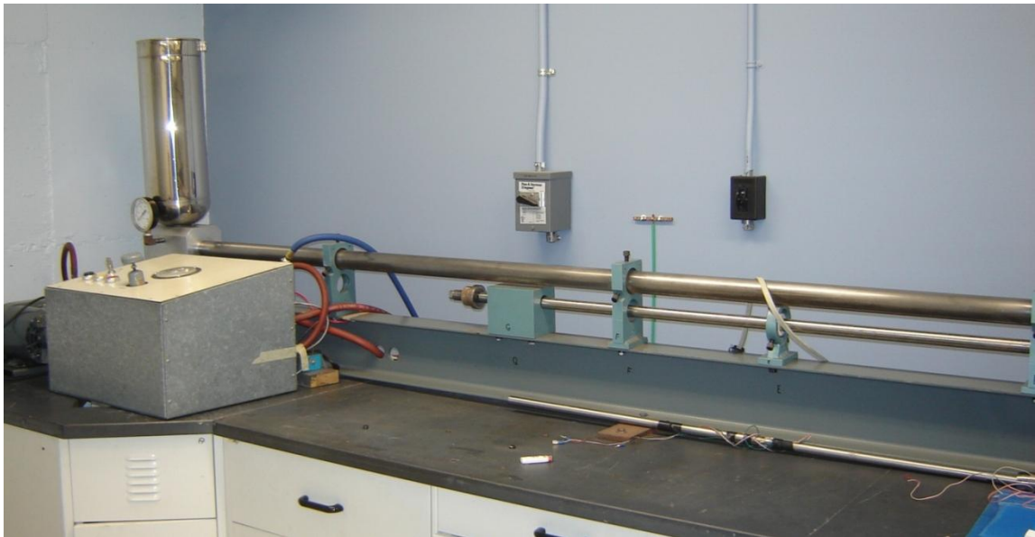
Figure 3.4: Image showing the control box, accumulator and firing chamber
