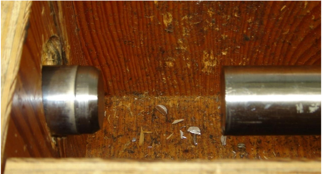
Figure 3.6: Sample placement on transmitted bar
