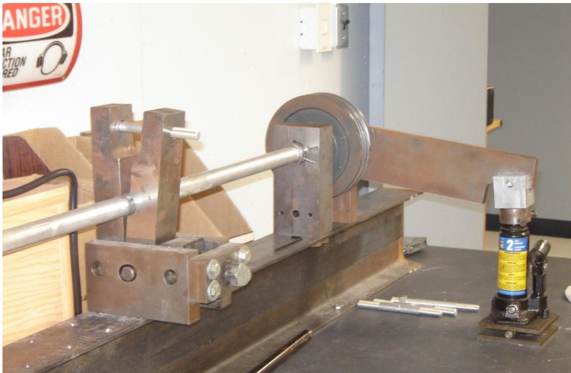
Figure 3.9: Clamping device and loading mechanism consisting of hydraulic jack and rotating wheel
