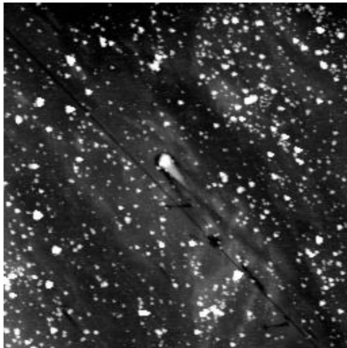
Figure 4.49: Region inside the white-etching bands (scan size 10\mu\text{m} \times 10\mu\text{m} )
