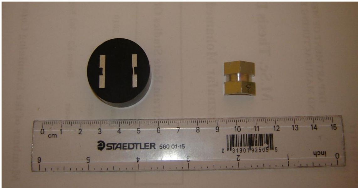
Figure 3.15: Specimen mounted from torsion loading experiments
