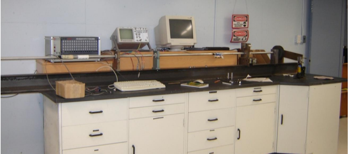
Figure 3.12: The TSHB showing incident bar, transmitted bar and data acquisition device
