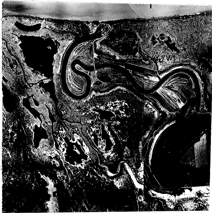
Plate XV. Air photograph showing truncation of the present northernmost bend of the Fort La Reine channel, 14-7W1.
