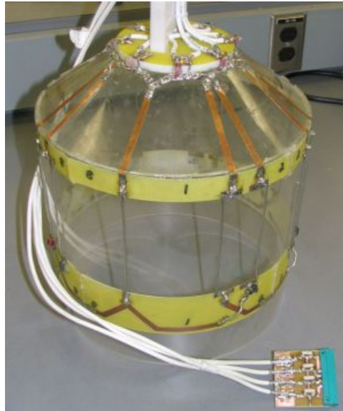
Figure 2.14 - Sample four-channel array coil designed by the author for human head imaging at 1.5T. This coil used eight different loops combined to form four channels [56].
