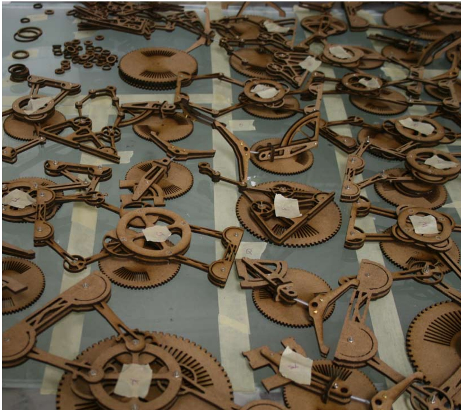
Gears were built for three specific types of movements. 'Anchor' gears adjust the land network from falling and touching other gears. 'Body' gears allow the land parcels to be maneuvered up, down and tilted and rotated. 'Arm' gears allow for lateral travel and lift. Worm gears would be used to control the movement of the structure.
