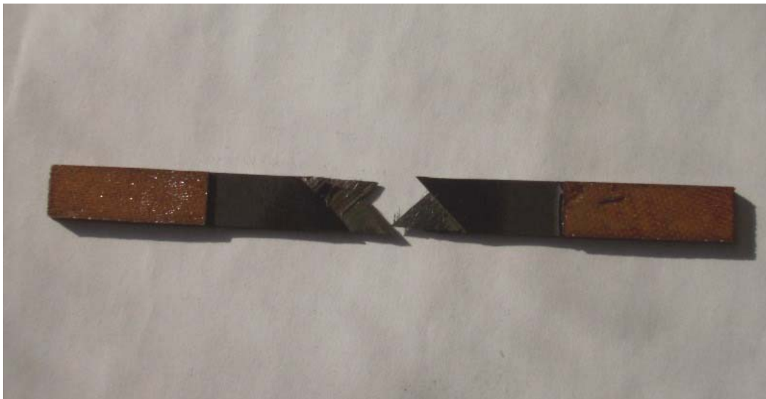
Figure 4.32: Fractured [\pm 45/90_2]_s sample after creep rupture testing at 180^{\circ}\text{C} and 90 % UTS
