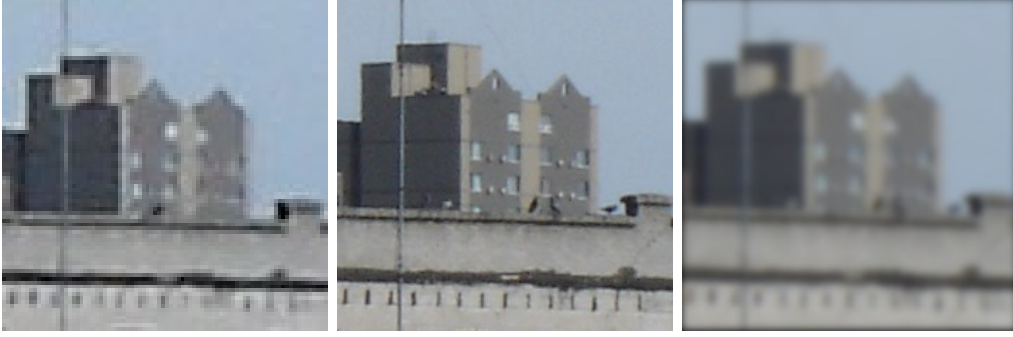
Figure 32: Scale space filtering. Left and middle images - images taken with a zoom factor 1 and 2.88, respectively, right image - middle image rescaled with factor \sigma = 2.88
