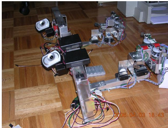
Figure 3.24: A pair of line crawling robots with mounted cameras
