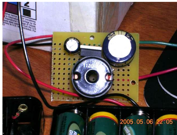
Figure 3.35: Completed buck regulator
