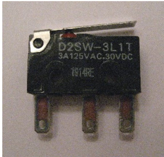
Figure 3.37: The microswitch used for contact sensors
