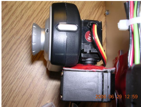
Figure 3.23: Creative NX Ultra mounted to position control servos connected to the robotic platform
