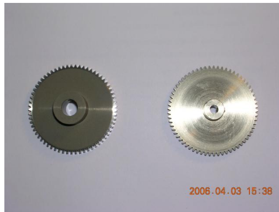
Figure 3.8: Spur gears used in line crawler power train
