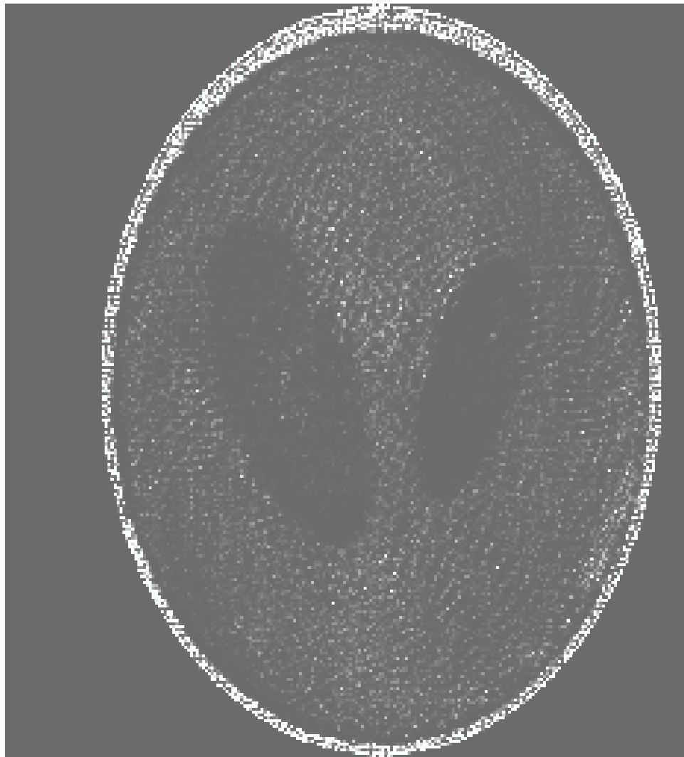
Figure 4.6: Reconstruction using view by round robin, MART at 256 \times 256 pixels, 4 processes.
