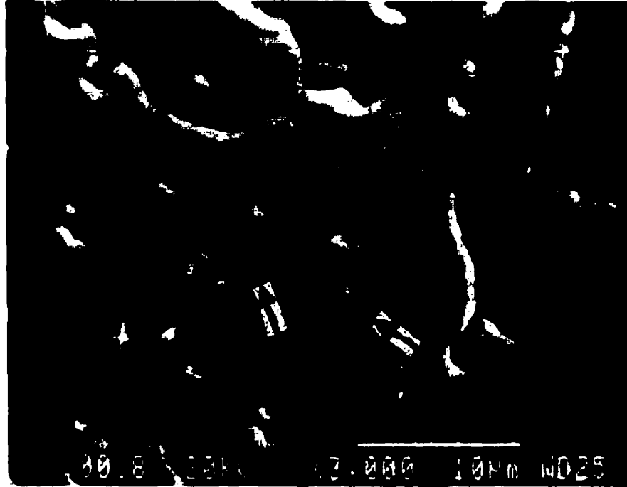
Figure 4.11 Secondary slip bands (SSBs) in 22μm-grained sample tested at a plastic strain of 2.1 \times 10^{-3}
