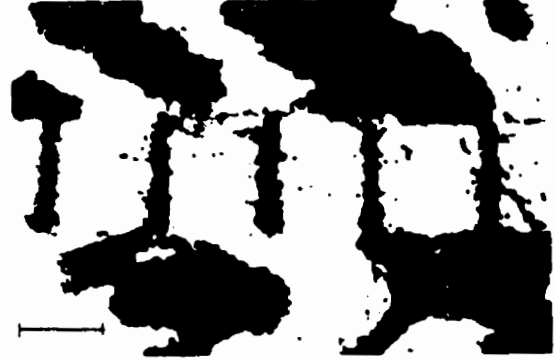
b) Range B : 6 \times 10^{-5} < \gamma_{pl} < 7.5 \times 10^{-5} . Primary dipolar walls of PSBs in matrix of primary dipole veins.
