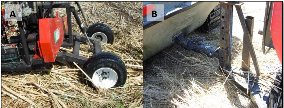
Figure 5.5 A) Harvester and tracked Argo caused only slight compaction of the litter and debris, but it rebounded quickly and left no permanent ruts. B) The front heavy design of the harvester weighed down the back of the Argo causing the adjustable hitch on the trailer to collect debris.
