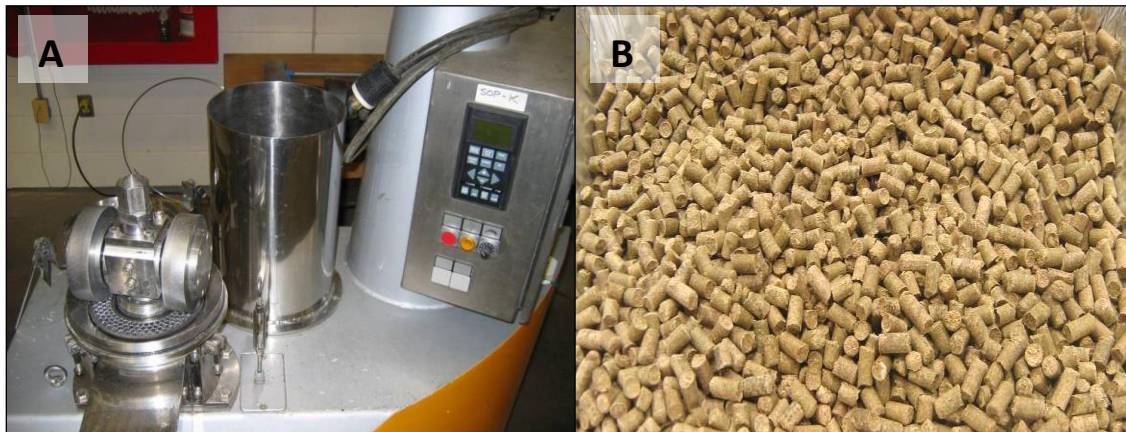
Figure 5.10. A) Pellet press used for pellet creation and analysis B) one of many batches of densified cattail pellets manufactured by Alberta Tech Futures.
