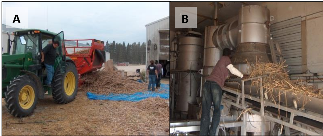
Figure 5.13. Gasification of cattails (2006). A) Bale shredding and B) feeding cattail biomass feedstock into gasifier unit for heat production.
