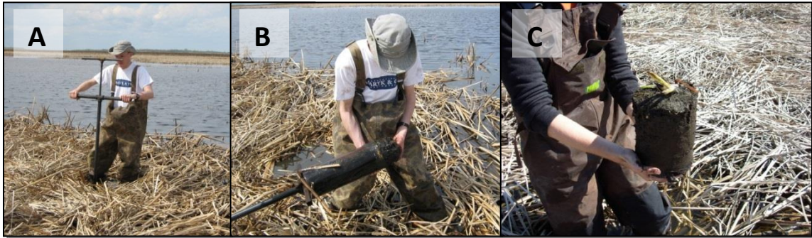
Figure 3.11. Belowground sampling in Netley-Libau Marsh. A) Coring for belowground plant samples, B) removing core from corer, and C) successful 6 inch diameter belowground core.
