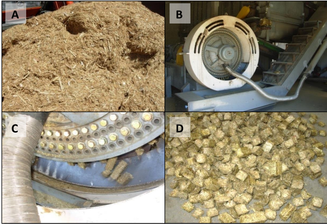
Figure 5.11. Cattail fuel cube production. A) Shredded cattail using bale shredder, B) modified hammermill, C) cattail/mixed marsh grass 1 inch x 1 inch fuel cubes being produced, D) cubes after packaging step ready for use in stoker boiler burners.
