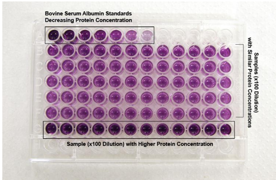
Figure 3.5 BCA assay microplate showing various shades of purple for different protein concentrations. Note the dark-to-light shades of purple on the top row signifying the decreasing protein concentrations of the bovine serum albumin standards. The middle five rows show samples at similar protein concentrations, followed by the last row showing a sample with higher concentrations.
