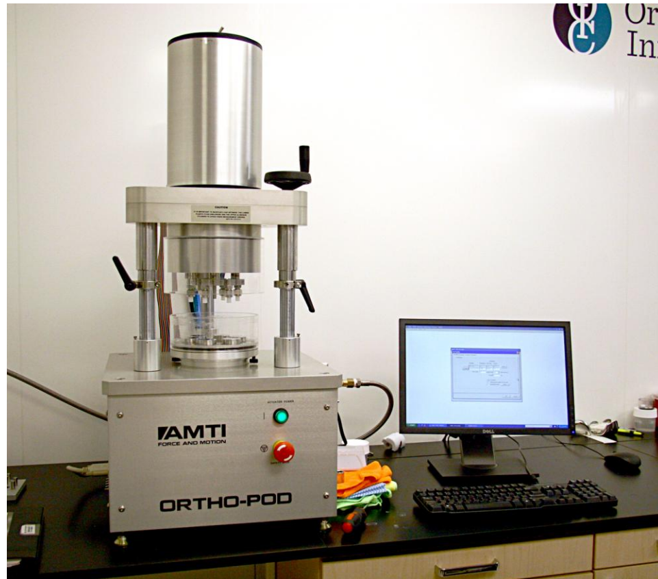
Figure 3.1: The AMTI OrthoPOD located in the Implant Simulator Laboratory at the Orthopaedic Innovation Centre.
