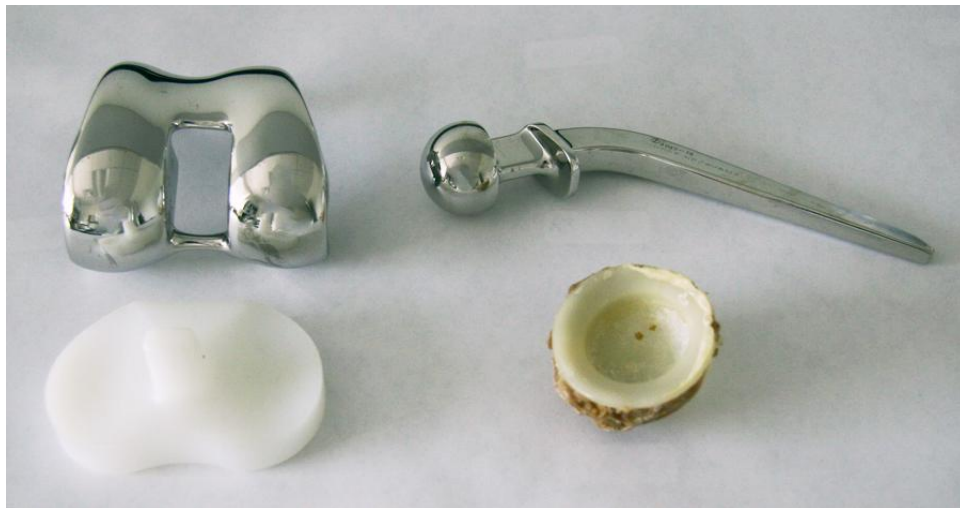
Figure 2.2: Image of a retrieved total knee and total hip replacement. The retrieved total knee replacement consists of a CoCr femoral component (left, top) and an ethylene oxide crosslinked PE tibial insert (left, bottom). The retrieved total hip replacement is shown with a CoCr femoral head and stem (right, top) with a crosslinked gamma sterilized PE acetabular insert (right, bottom). Note the characteristic yellowing and delamination of the gamma sterilized acetabular insert (right, bottom) in comparison to the ethylene oxide sterilized tibial insert (left, bottom).
