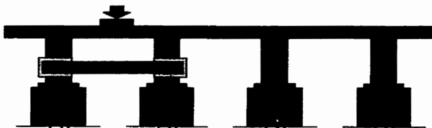
Figure 6-3: End Restraint for Slab C-2 Test
