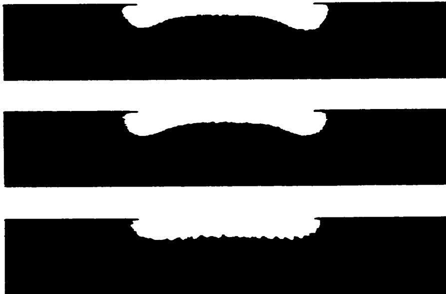
Figure 5-5. Simulation results showing the trenching phenomenon for and its changes with \lambda . The hole with is 400\mu\text{m} and the reaction probability was set to 0.01.
