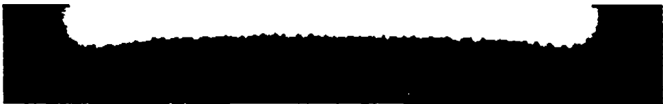
Figure E-17. Experimental and simulation results for a 1000µm hole. The actual trench depth is 4.9µm versus 7µm for simulated result.
