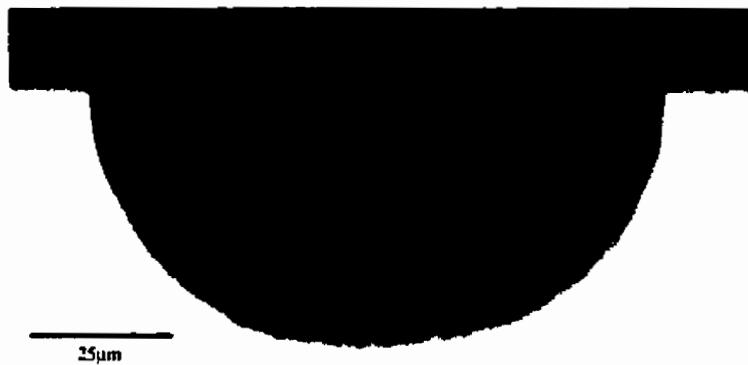
Figure 4-9. The etch profile for small size mask openings.
