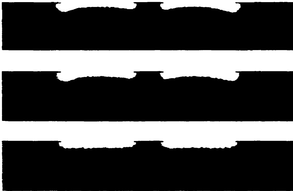
Figure 5-6. Simulation results showing the loading effect for two neighbor holes. The hole diameters are 200\mu\text{m} each, the distance between them is 100\mu\text{m} , and the reaction probability was set to 0.01.
