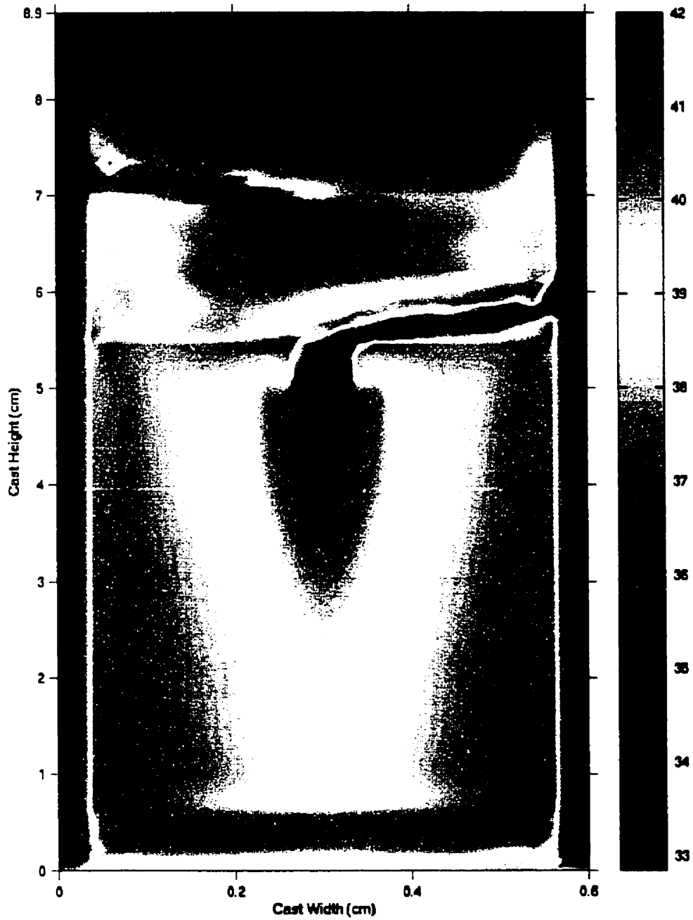
Figure 3.15 Fully solidified Al-38wt%Cu alloy at R = 11 cm/hr, concentration of solid (wt%Cu)
