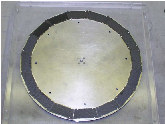
Figure 3.3: On the left is a picture of the production target wheel showing 16 carbon targets at the outer diameter of the wheel. On the right is a picture of the vacuum housing for the rotating target wheel. The beam from ATLAS enters from the left and strikes the target in the upper section of the cylindrical vacuum chamber before entering the magnetic quadrupoles (in blue).
