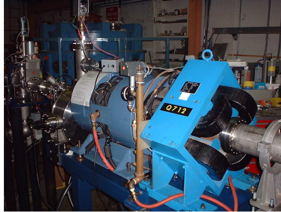
Figure 3.4: The magnetic quadrupole triplet. Reaction products which emerge from the target on the left travel through a combination of a doublet, then a singlet, before entering the velocity filter off to the right.
