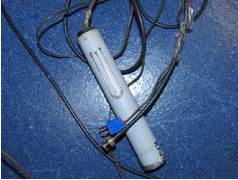
Fig. 3.5 One section of the new multilevel TDR probe
