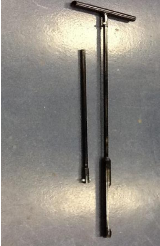
Fig. 3.8 A new soil auger designed for creating access holes in the soil.
