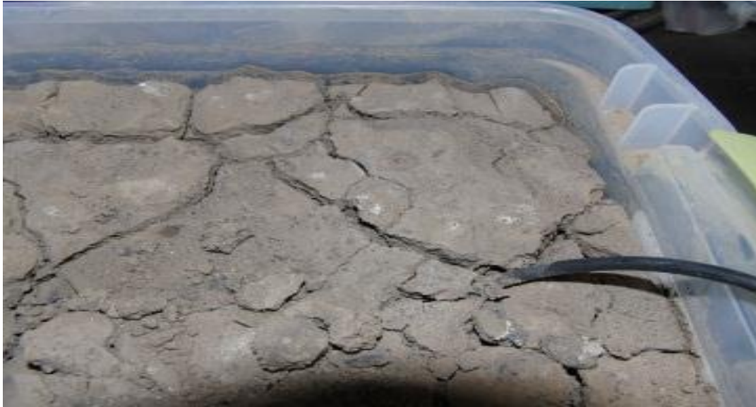
Fig. 5.1 Cracks in the soil creating air gap.
